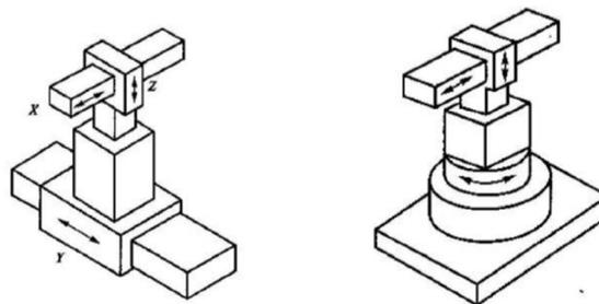
Figure 1. Cartesian and Cylindrical Coordinate Robots.
