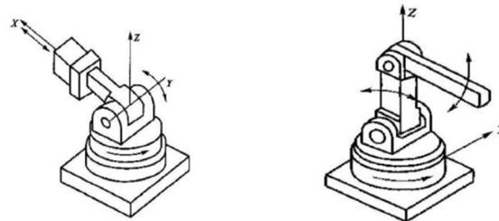
Figure 2. Spherical and Articulated Coordinate Robots.
