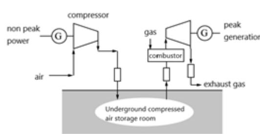
**Figure 2.** Schematic diagram of compressed air energy storage.
