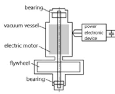
**Figure 3.** Schematic diagram of flywheel energy storage
