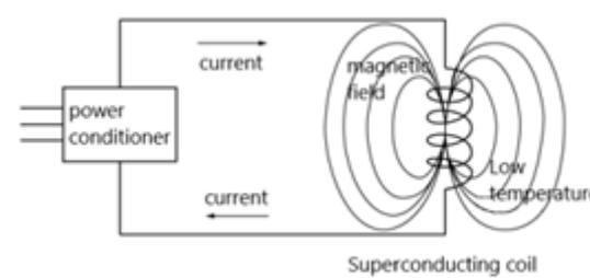
**Figure 5.** Sketch map of superconducting magnetic energy storage
