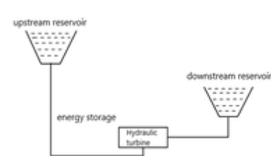
**Figure 1.** Schematic diagram of pumped storage.
