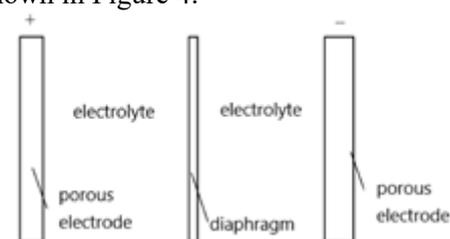
**Figure 4.** Schematic diagram of capacitor energy storage
