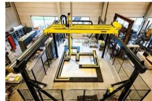
Figure 6. The printer for Contour Crafting.
