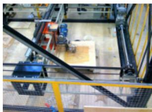
Figure 3. The printer for Concrete Printing.
