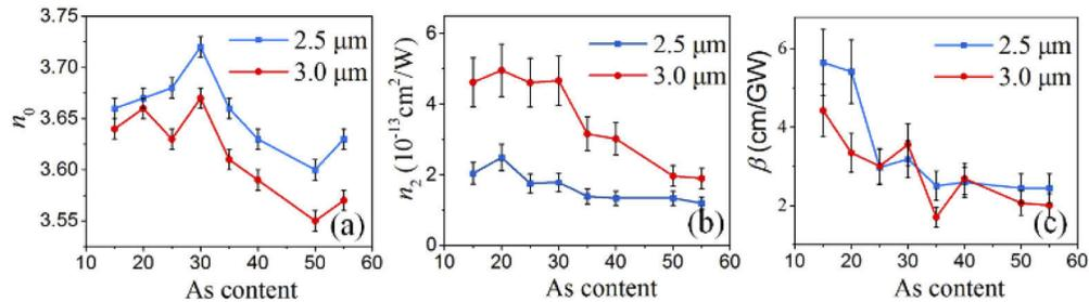
**Fig. 3.** (a) Linear refractive index, (b) nonlinear refractive index and (c) two-photon absorption coefficient as a function of As content in mol% at 2.5  $\mu\text{m}$  (blue) and 3.0  $\mu\text{m}$  (red).
