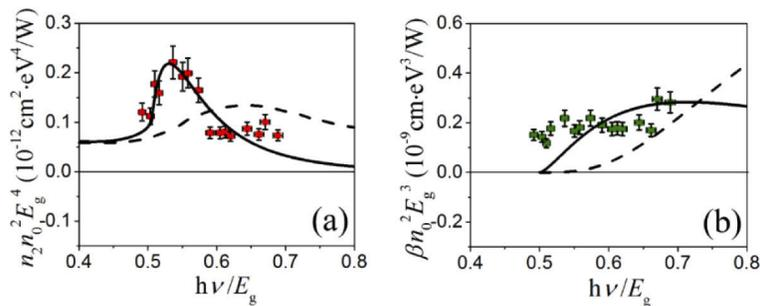
**Fig. 5.** (a). The behavior of normalized  $n_2$  as a function of  $h\nu/E_g$ . (b) The behavior of normalized two photon absorption as a function of  $h\nu/E_g$ . The squares are the experimental data, the solid line are the fitting curves based on Sheik-Bahae's model and the dashed lines are Dinu's model.
