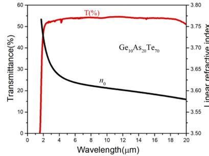
**Fig. 2.** Optical transmittance spectrum and linear of refractive index dispersion for  $\text{Ge}_{10}\text{As}_{20}\text{Te}_{70}$  glass.
