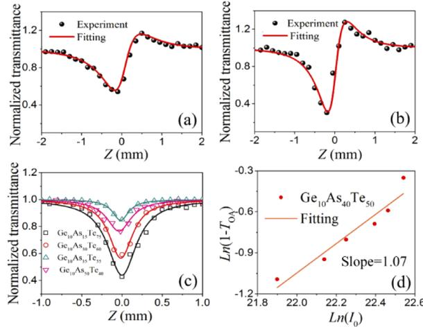
**Fig. 1.** Closed-aperture Z-scans measurement and fittings for  $\text{Ge}_{10}\text{As}_{20}\text{Te}_{70}$  at 2.5  $\mu\text{m}$  (a) and at 3.0  $\mu\text{m}$  (b). (c) The open aperture measurement and the fitting for four compositions. (d) The linear fitting of  $\ln(1-T_{OA})$  vs peak irradiance  $\ln(I_0)$ . The slope of the fitting line determines the two-photon absorption.
