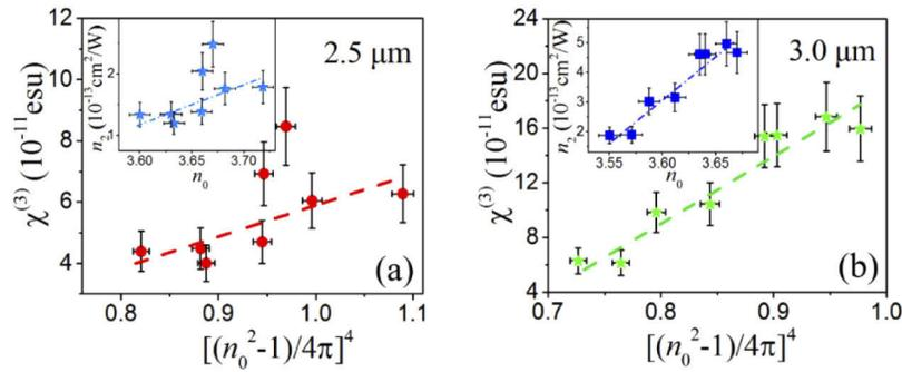
**Fig. 4.** Variation of the nonlinear susceptibility versus  $(n_0^2-1)/4\pi$ . Dashed lines are the theoretical fitting based on Eq. (5) at (a) 2.5  $\mu\text{m}$ , and (b) 3.0  $\mu\text{m}$ . The inset is the dependence of experimental  $n_2$  on  $n_0$ .
