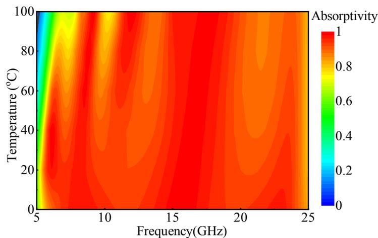
Fig. 7. Absorption spectrum of the absorber at different temperatures.
