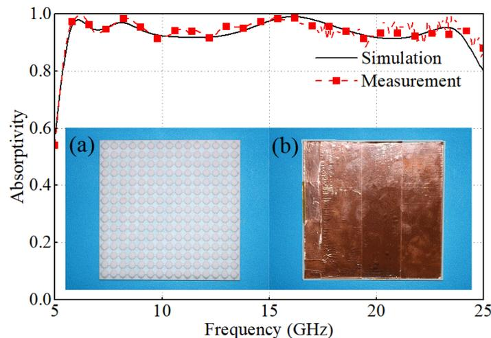
Fig. 5. Simulated and measured absorption spectra of the proposed absorber. Inset: Photo of absorber prototype with  $15 \times 15$  elements. (a) Top view and (b) bottom view.
