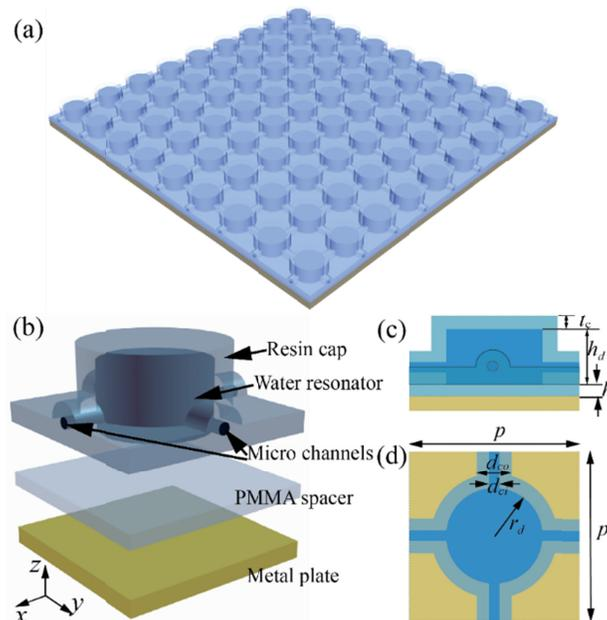
Fig. 1. (a) Schematic of the cylindrical-water-resonator-based ultra-broadband absorber. (b) Exploded view of the unit cell of the absorber. Each part of the unit cell is arranged layer-by-layer. (c) Side view and (d) top view of the unit cell. The geometrical parameters are as follows:  $p = 11.4$  mm,  $r_d = 3.2$  mm,  $h_d = 3.8$  mm,  $t_c = 1$  mm,  $h_s = 0.8$  mm,  $d_{ci} = 0.6$  mm, and  $d_{co} = 2.2$  mm.
