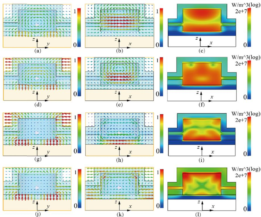
Fig. 4. Simulated vector field distribution in the absorber. (a, d, g, j)  $E$ -field in  $xoz$  plane for  $f_1$ ,  $f_2$ ,  $f_3$ , and  $f_4$  of 6.07, 8.1, 16.19, and 23.45 GHz, respectively. (b, e, h, k)  $H$ -field in  $yo$ z plane for  $f_1$ ,  $f_2$ ,  $f_3$ , and  $f_4$  of 6.07, 8.1, 16.19, and 23.45 GHz, respectively. (c, f, i, l) Power-loss density in  $xoz$  plane for  $f_1$ ,  $f_2$ ,  $f_3$ , and  $f_4$  of 6.07, 8.1, 16.19, and 23.45 GHz, respectively.
