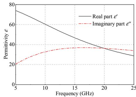
Fig. 2. Permittivity of water at 5–25 GHz obtained using Debye model.
