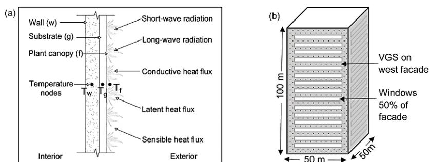
Fig. 1. (a) Heat fluxes account in the VGS model (b) Schematic diagram of EnergyPlus building model
