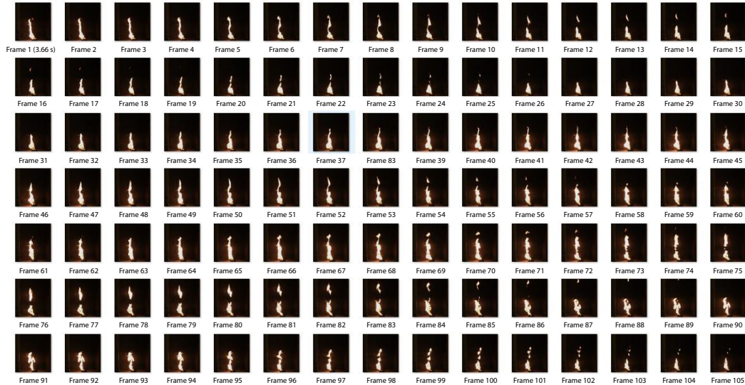
Figure 3. Test T10h1 at time 3.66-4.08 seconds (duration of 0.42 second for 105 frames), frame interval 0.004 second captured using a high-speed camera
