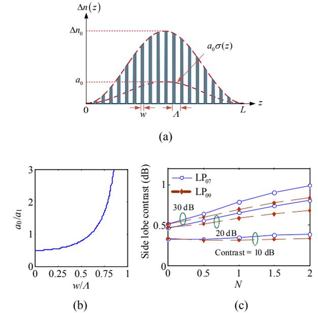
Fig. 7 Characteristics of a typical laser-written apodized LPFG: (a) index profile, (b) dependence of the ratio  $a_0/a_1$  on the duty cycle  $w/A$  of the index modulation, and (c) dependence of the contrast of the most significant side lobe on the apodization profile and the mode order, calculated for  $a_0/a_1 = 0.5$  and the resonance contrasts 10 dB, 20 dB, and 30 dB.
