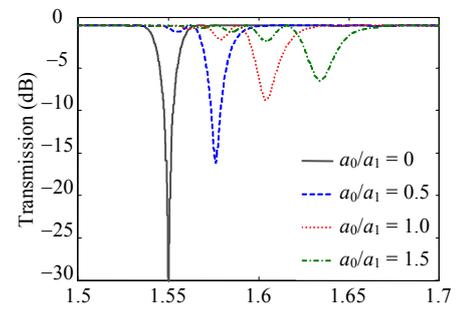
Fig. 3 Transmission spectra of a 60-mm-length raised-cosine apodized LPFG calculated for four different values of  $a_0/a_1$ : 0, 0.5, 1.0, and 1.5, where  $a_1$  is fixed to ensure complete rejection at the nominal wavelength  $1.55 \mu\text{m}$ .
