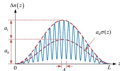
Fig. 2 A raised-cosine ( $N = 2$ ) apodization profile showing the dc and ac components.
