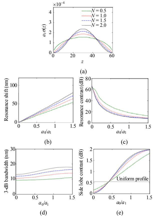
Fig. 5 Effects of the ratio  $a_0/a_1$  on the transmission characteristics of (a) four 60-mm apodized LPFGs with  $N = 0.5, 1.0, 1.5,$  and  $2.0$ , (b) the resonance wavelength shift, (c) the contrast of the rejection band, (d) the 3-dB bandwidth of the rejection band, and (e) the contrast of the most significant side lobe.
