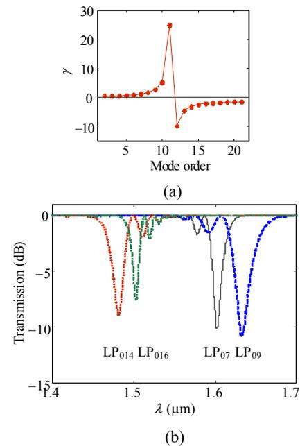
Fig. 6 Effects of the cladding-mode orders: (a) modal dispersion factor of the first twenty cladding modes at  $1.55 \mu\text{m}$  and (b) transmission spectra of four 60-mm-length raised-cosine apodized LPFGs with  $a_0/a_1 = 1.0$ , which are designed for operation with the  $\text{LP}_{07}$ ,  $\text{LP}_{09}$ ,  $\text{LP}_{014}$  and  $\text{LP}_{016}$  cladding modes, respectively.
