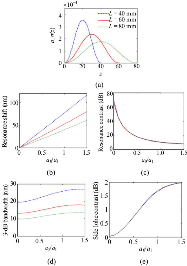
Fig. 4 Effects of the ratio  $a_0/a_1$  on the transmission characteristics of (a) three raised-cosine apodized LPFGs with  $L = 40$  mm, 60 mm, and 80 mm, (b) the resonance wavelength shift, (c) the contrast of the rejection band, (d) the 3-dB bandwidth of the rejection band, and (e) the contrast of the most significant side lobe.
