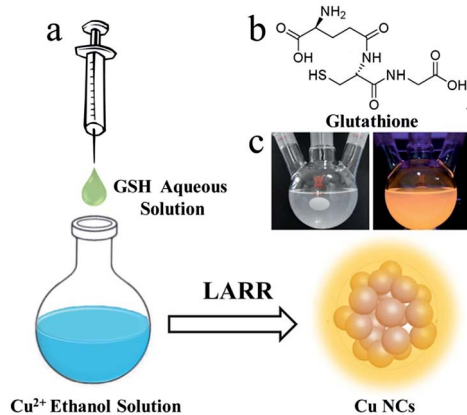
Fig. 1 (a) Schematic illustration of the synthesis of Cu NCs using the LARR method. (b) Structure of GSH. (c) Optical images of a solution of Cu NCs under daylight and UV light.
