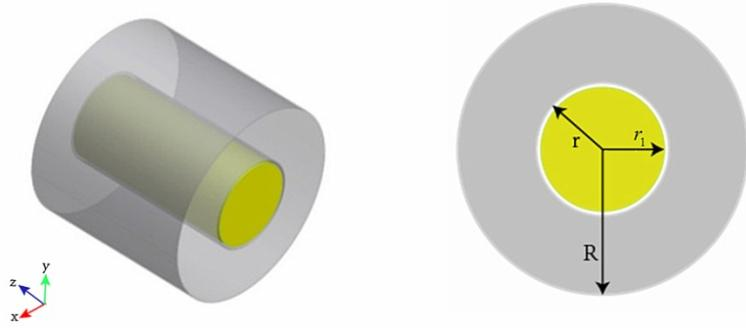
Fig. 1. Schematic illustration of the metal-dielectric hybrid nanodisk.
