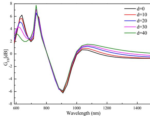
Fig. 10. Far-field forward-to-backward directionality  $G_{FS/BS_{min}}$  for electric dipole excitation.
