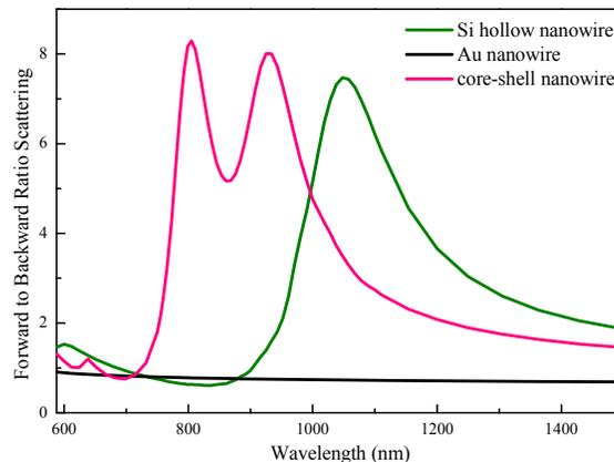
Fig. 9. Forward/backward ratio scattering spectra of the Si hollow nanodisk, Au nanodisk, and core-shell nanodisk with  $H = 220$  nm,  $R = 120$  nm,  $r = 50$  nm,  $r_1 = 48$  nm.
