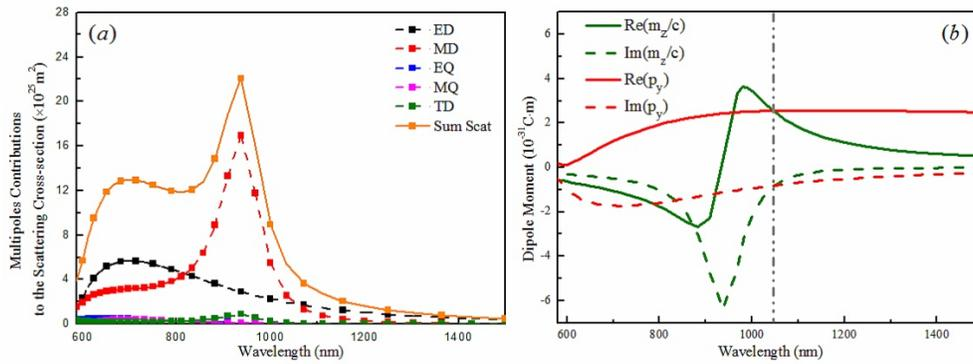
Fig. 2. (a) Multipole contributions to the scattering cross-section and (b) Real and imaginary components of the electric and magnetic moments of individual silicon hollow nanodisk with  $H = 220 \text{ nm}$ ,  $R = 120 \text{ nm}$ ,  $r = 50 \text{ nm}$ .
