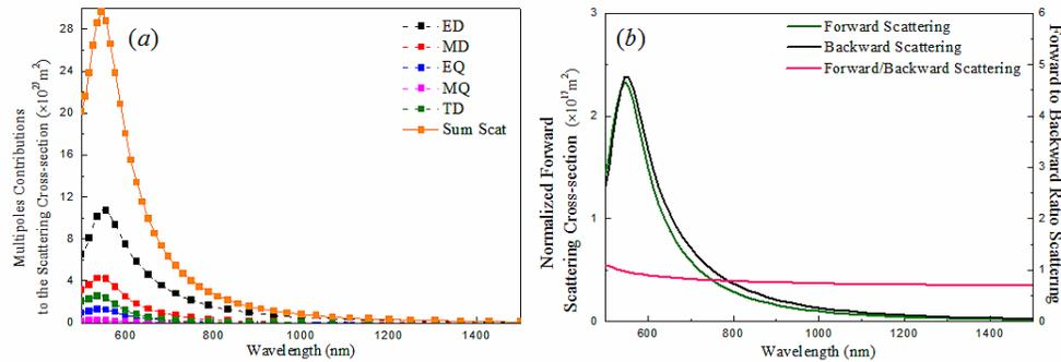
Fig. 4. (a) Multipole contributions to the scattering cross-section and (b) Forward and backward scattering and forward/backward ratio scattering spectra of the individual Au nanodisk with  $H = 220 \text{ nm}$ ,  $r = 48 \text{ nm}$ .
