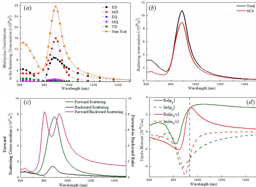
Fig. 6. (a) Multipole contributions to the scattering cross-section, (b) Comparison of the total total scattering cross-section with SCS, (c) Forward and backward scattering and forward/backward ratio scattering spectra, and (d) Real and imaginary components of the electric and magnetic moments of the core-shell nanodisk. The core nanodisk is made of gold of  $r_1 = 48$  nm and the shell is the  $n = 3.5$  dielectric with  $H = 220$  nm,  $R = 120$  nm,  $r = 50$  nm.
