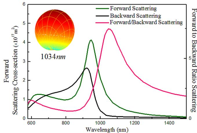
Fig. 3. Forward and backward scattering and forward/backward ratio scattering spectra for the individual hollow silicon nanodisk with  $H = 220 \text{ nm}$ ,  $R = 120 \text{ nm}$ ,  $r = 50 \text{ nm}$ .
