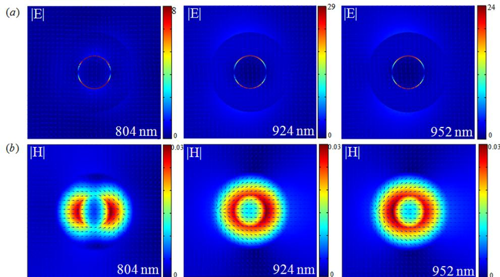
Fig. 7. Spatial profiles: (a) Electric field and (b) Magnetic field at the wavelengths of FS/BS<sub>max</sub>
