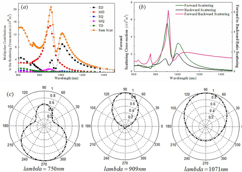
Fig. 5. (a) Multipole contributions to the scattering cross-section, (b) Forward and backward scattering and forward/backward ratio scattering spectra, and (c) Scattered field pattern of core-shell nanodisk. The core nanodisk is made of gold of  $H = 220 \text{ nm}$ ,  $r_1 = 50 \text{ nm}$ ,  $r = 50 \text{ nm}$  and the shell is the  $n = 3.5$  dielectric with radius  $R = 120 \text{ nm}$ .
