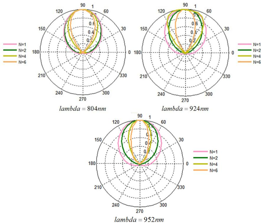
Fig. 11. Scattering pattern by an array of nanoantennas with  $N = 1, 2, 4, 6$ .
