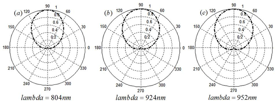
Fig. 8. Scattered field pattern of the core-shell nanodisk with  $H = 220$  nm,  $R = 120$  nm,  $r = 50$  nm,  $r_1 = 48$  nm calculated at the wavelength 804 nm and 924 nm. The angle of  $90^\circ$  ( $270^\circ$ ) corresponds to the forward (backward) direction.
