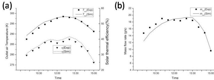
Fig. 2: Comparison between the simulations and experimental data for (a) Air mass flow rate; (b) Outlet air temperature and solar efficiency
