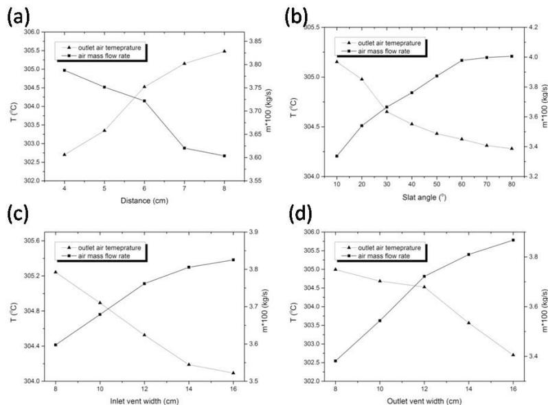
Fig. 4: Air mass flow rate and outlet air temperature as a function of: (a) slat position (distance between the slats and inner wall); (b) slat angles; (c) the area of the inlet vent; (d) the area of the outlet vent in transition season mode.
