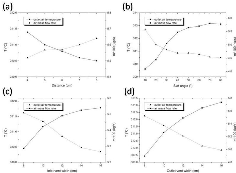
Fig. 3: Air mass flow rate and outlet air temperature as a function of: (a) slat position (distance between the slats and inner wall); (b) slat angles; (c) the area of the inlet vent; (d) the area of the outlet vent in summer mode.
