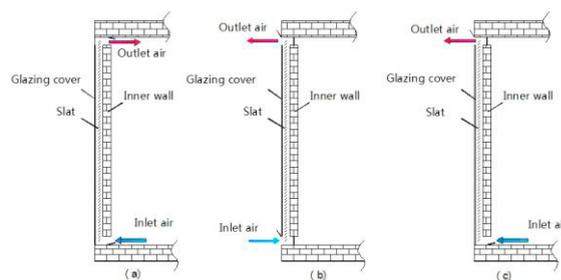
Fig. 1: Schematics of Trombe wall with venetian blind structure: (a) winter mode; (b) summer mode; (c) transition season mode.
