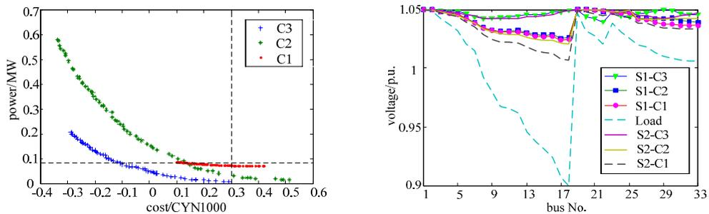
Fig. 6. Pareto front of different cases and the voltage of 33-bus distribution grid in different scenarios
