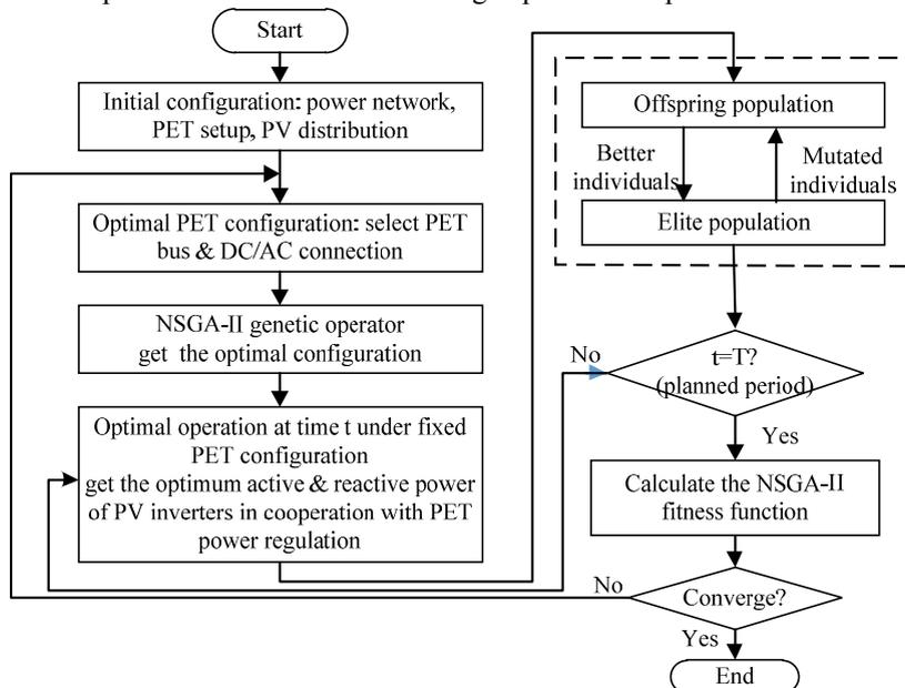
Fig 2. Flowchart of the proposed coordinated optimization algorithm
