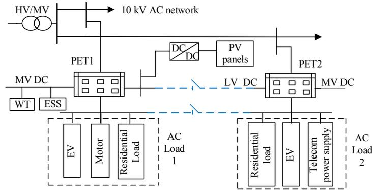
Fig. 1. PET installed in the MV/LV distribution grid with DC/AC generation and loads
