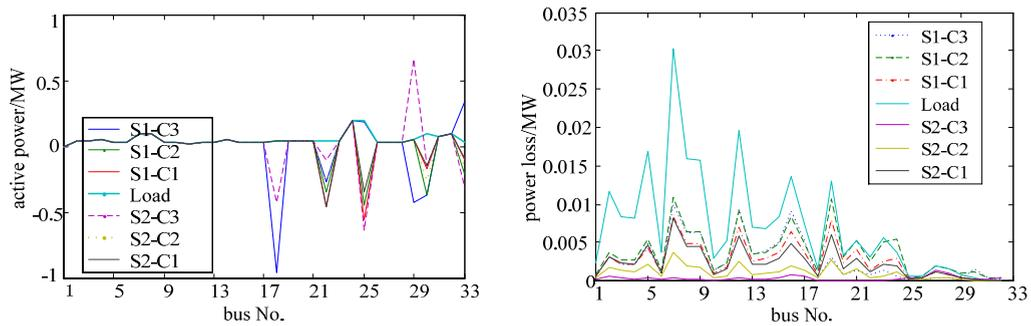
Fig. 7. Active power and power losses of the 33-bus distribution grid in different scenarios
