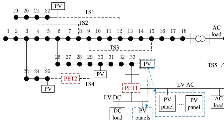
Fig 3. 33-bus distribution network with PV integration and updated PET bus
