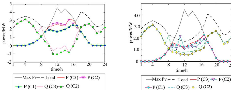
Fig. 4. Daily power profiles of load and PV generation in the scheme 1 and scheme 2
