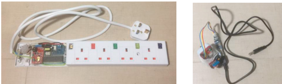
Fig. 3. The appearance of the Prototype for a) IS Strip; and b) IS Strip Receiver
