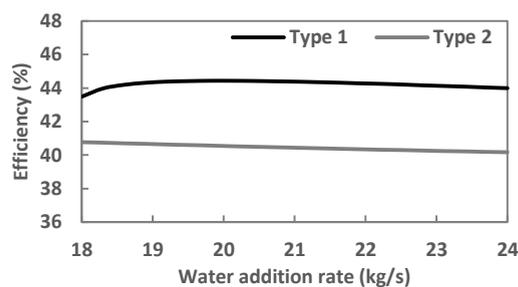
Fig.3. Variation of efficiency with water addition rate
