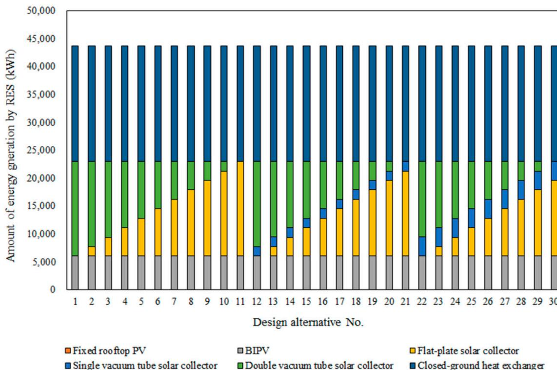
Figure 7. Amount of energy generation per RES in each design alternative.
