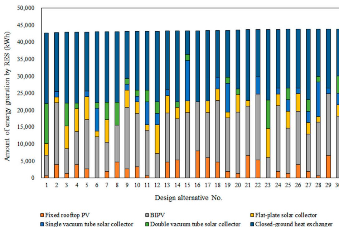
Figure 5. Amount of energy generation per RES in each design alternative.
