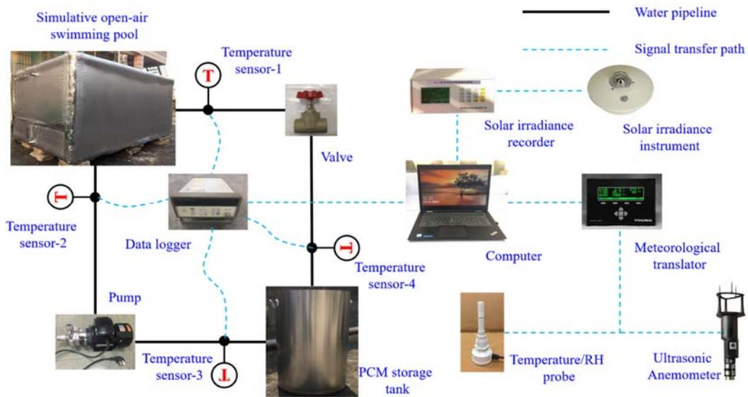
**Figure 2.** Schematic diagram of the constructed experimental setup.
