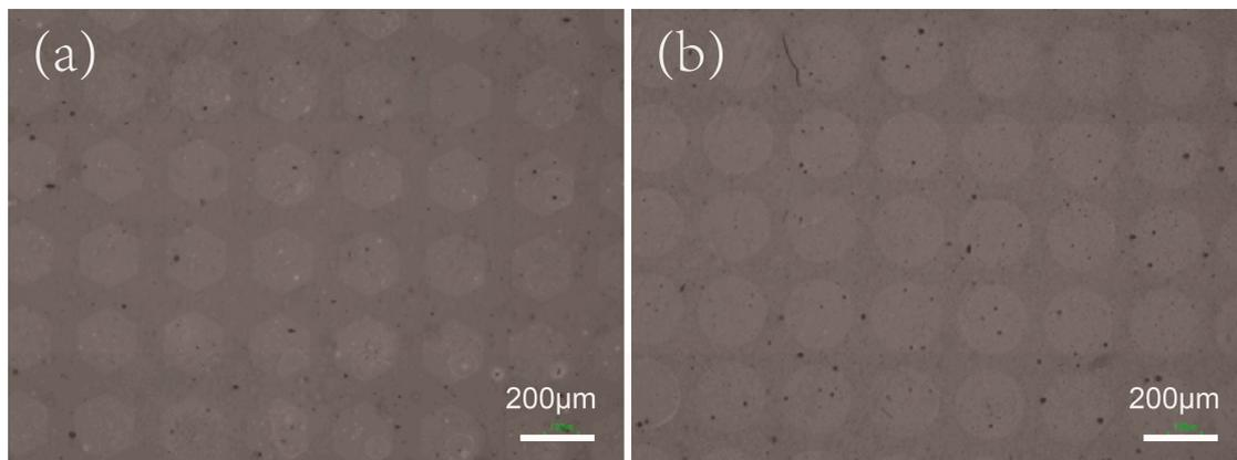
**Figure 2.** Optical microscope images of the frequency selective surface (FSS) with the patterned hexagonal (a) or circular (b) Au NP monolayer.
