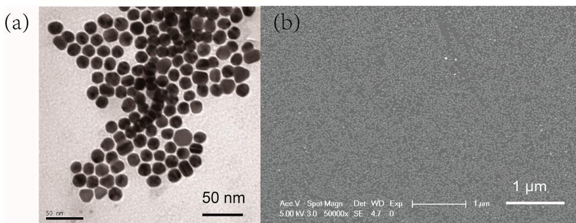
**Figure 3.** (a) Transmission Electron Microscope image of gold nanoparticle and (b) Scanning Electron Microscope image of gold nanoparticle monolayer on the PET substrate.
