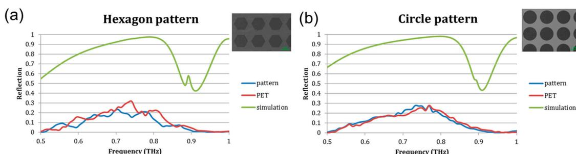
**Figure 4.** Time-domain spectroscopy (TDS) measurement and simulation results of FSSs made with an Au NP monolayer with hexagonal (a) and circular (b) patterns.
