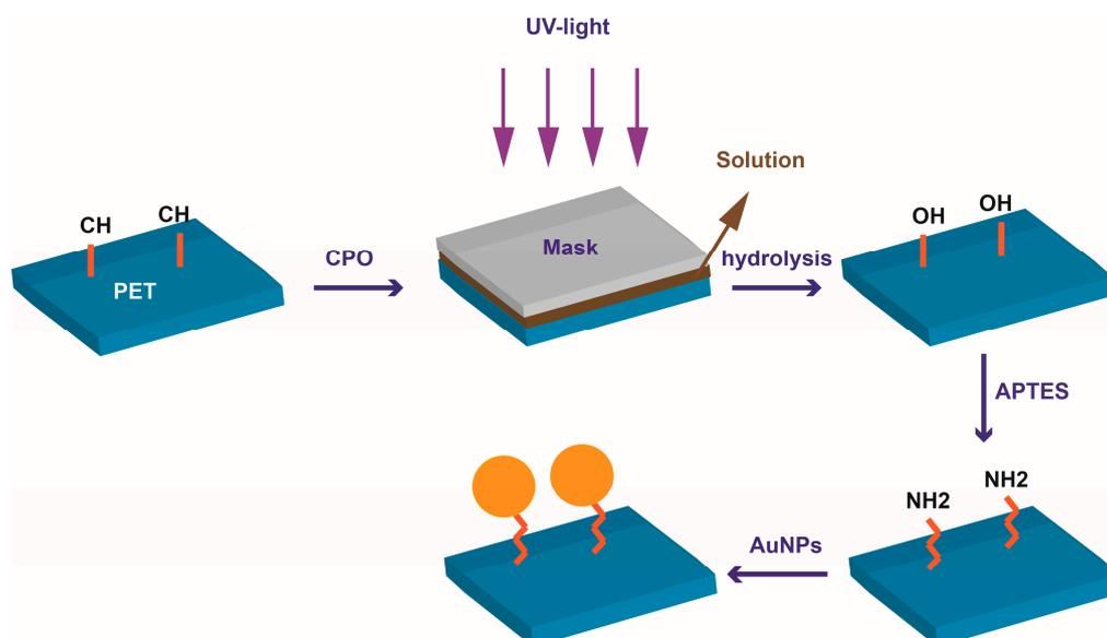
**Figure 1.** Schematic diagram depicting application of the confined photocatalytic oxidation (CPO) based self-assembled gold nanoparticle (Au NP) monolayer surface pattern on flexible polyethylene terephthalate (PET) substrate.
