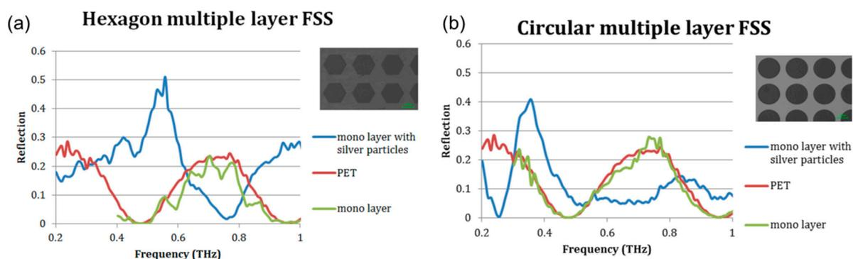
**Figure 5.** TDS measurements of FSSs made of silver-isolated islands with hexagonal (a) and circular (b) shapes.
