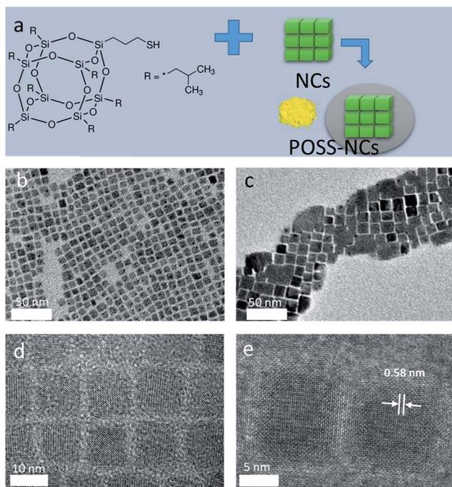
Fig. 1 (a) Structure of a thiol-functionalized POSS, with a schematic diagram illustrating the POSS coating process for preparation of perovskite NC powders. (b and c) TEM images of CsPbBr<sub>3</sub> perovskite NCs before and after POSS coating. (d and e) HRTEM images of CsPbBr<sub>3</sub> perovskite NCs before and after POSS coating. A characteristic lattice plane distance of 0.58 nm for cubic phase CsPbBr<sub>3</sub> perovskite is indicated in (e).
