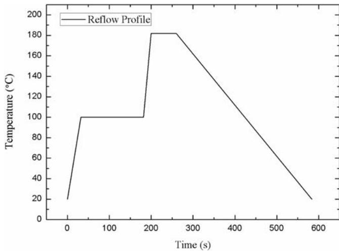
Fig. 1. Reflow profile for Cu/Sn-58Bi/Cu solder joints.
