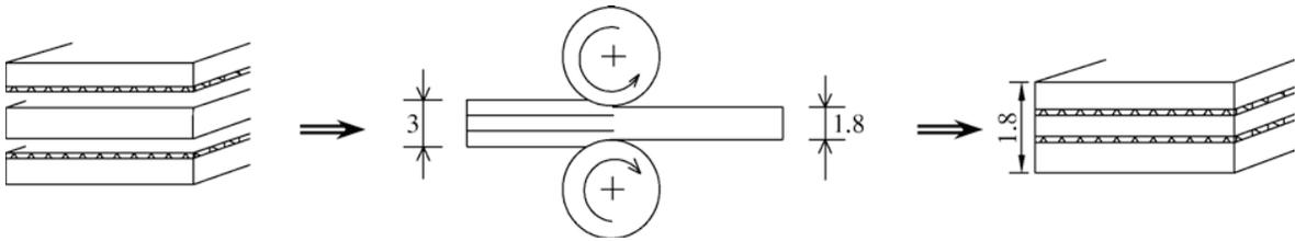
Fig. 3. Schematic illustrations of co-warm rolling process [11].
