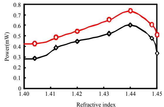
Fig.4 Dependence of the sensor output on the surrounding refractive index for two parallel over-coupled gratings with an offset distance of 0 mm(lower curve) or 5 mm (upper curve).
