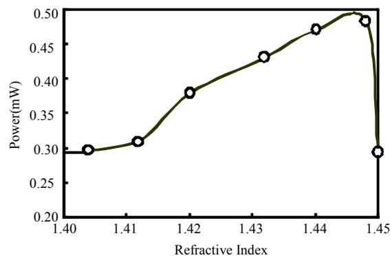
Fig. 2 Dependence of the sensor output on the surrounding refractive index for two parallel CO<sub>2</sub>-laser written LPFGs with an offset distance of 10 mm.
