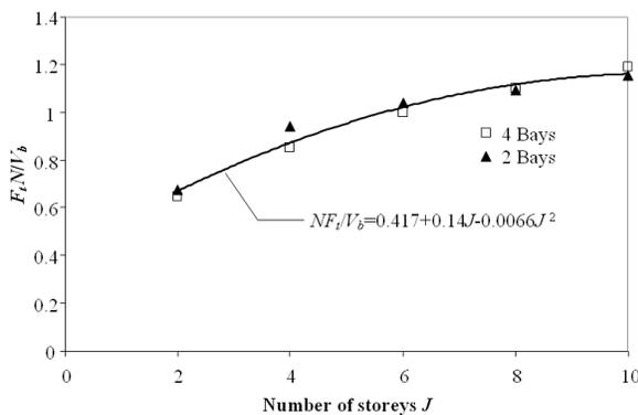
Fig. (8). Normalized tensile force in the critical tie.
