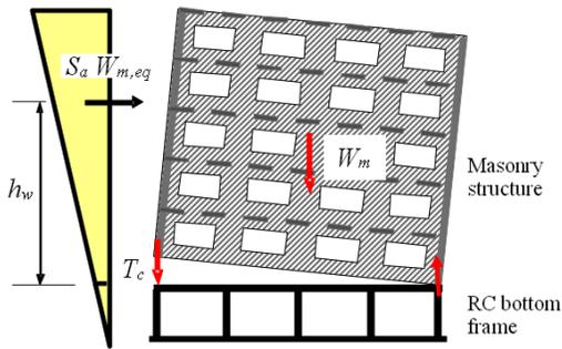
Fig. (10). Free body diagram of the masonry structure above the RC bottom frame.
