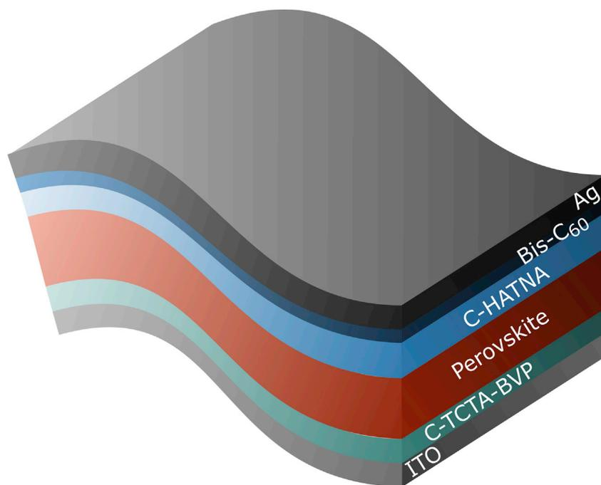
**Figure 1. A Schematic of a Flexible Planar p-i-n Perovskite Solar Cell Using Low-Temperature Processed All-Crosslinked Charge Extraction Layers**
