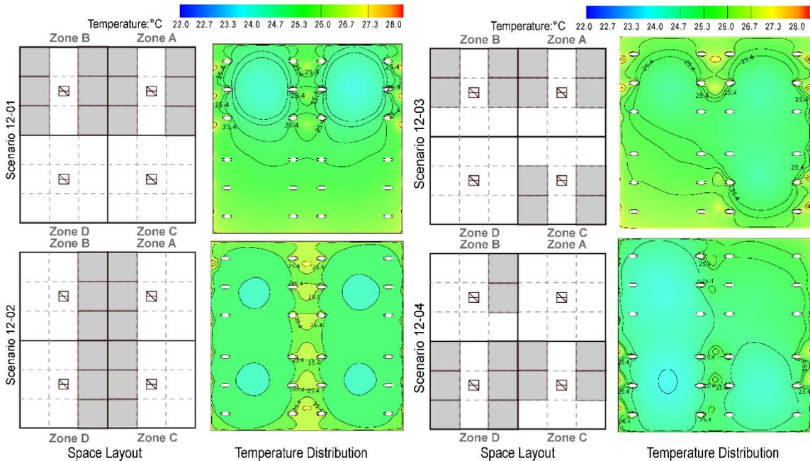
Fig. 3. Space layout and temperature distribution in the four scenarios of case 12
