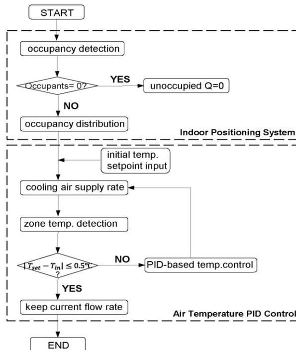
Fig.2. The supervised demand-driven control algorithm
