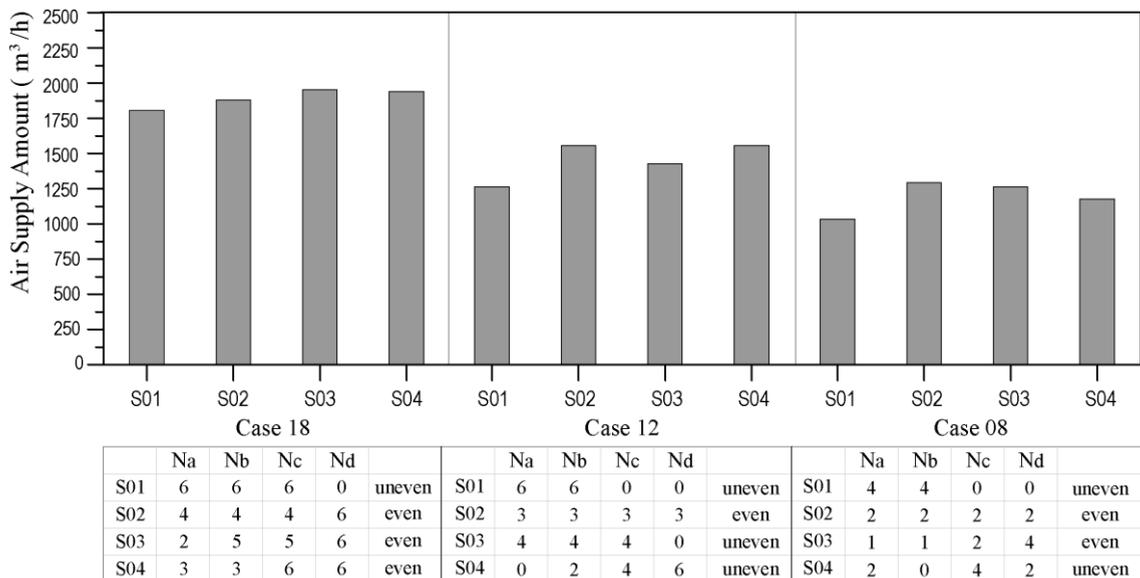
Fig. 4. The air supply amount and the number of occupants in each scenario of three cases.
