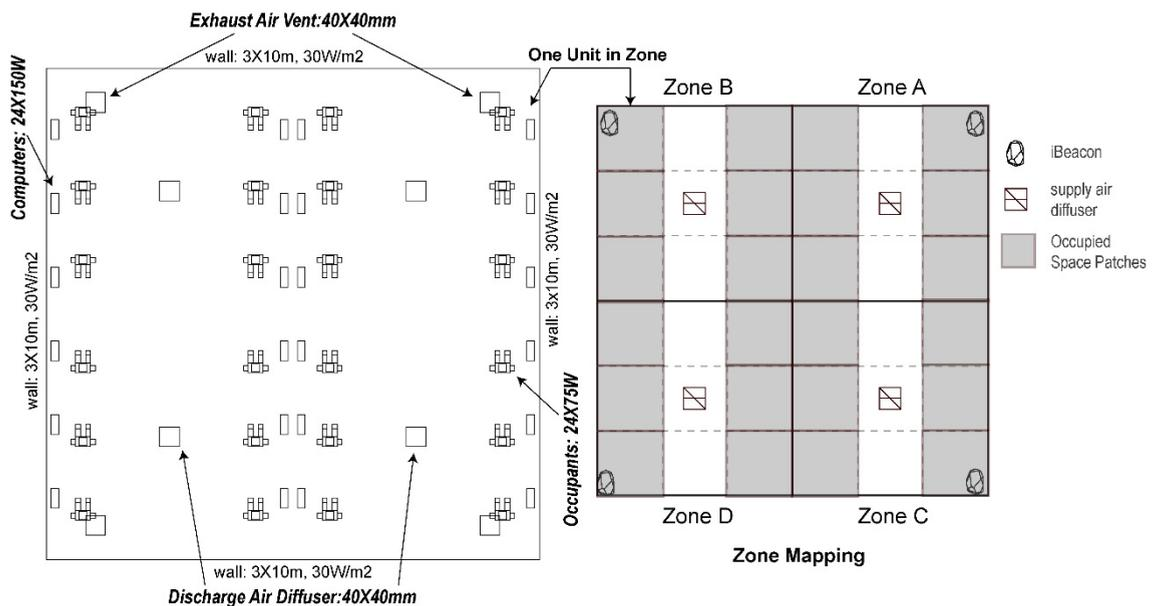
Fig.1. The model specifications and zone mapping of simulation space
