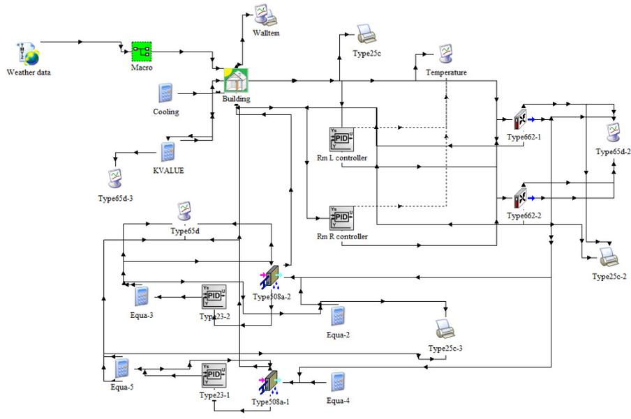
Fig. 4. Zonal temperature control platform
