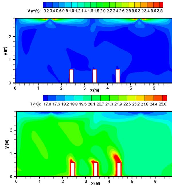
Fig. 3. Contour of velocity and temperature in x cut plane ( $x=1.5\text{m}$ )
