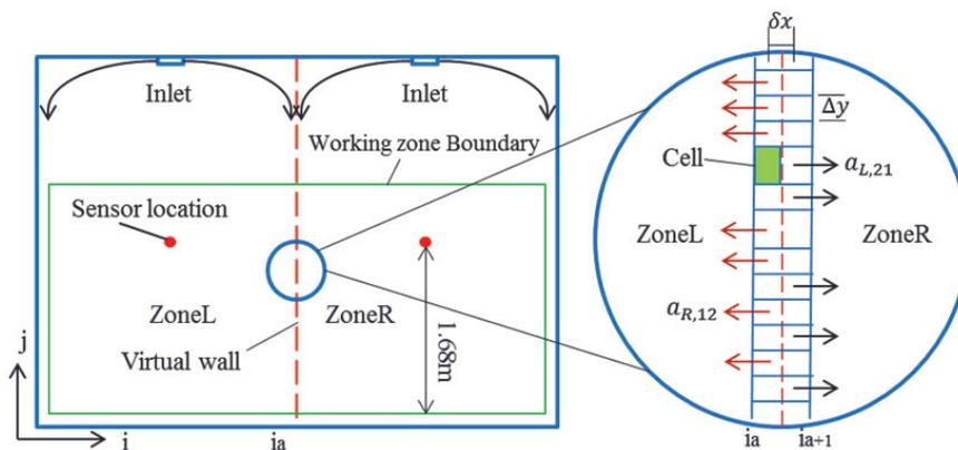
Fig. 1. Calculation heat transfer between virtual walls
