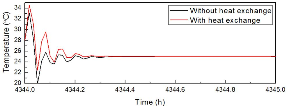
Fig. 5. The response of the controller with and without heat exchange added into the control platform (Left room)
