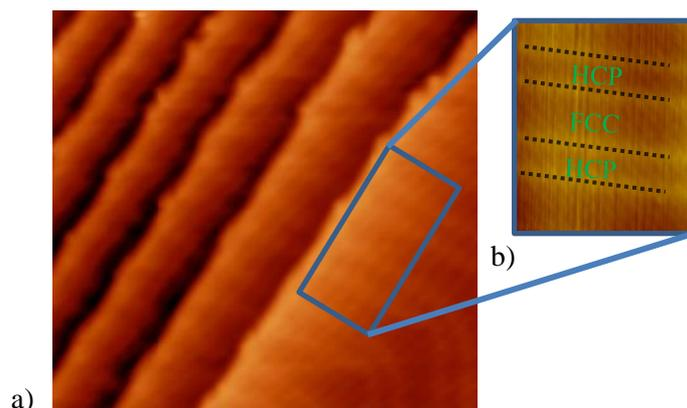
Figure 1. (a) STM topography image of Au (111) at  $I_t = 20$  nA,  $V_{bias} = 1$  V; and (b) Magnified STM image of HCP domains and FCC domains of Au (111).
