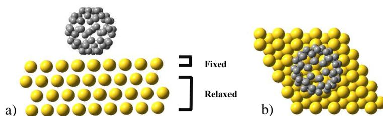
Figure 3. (a) Side view of adopted model for  $C_{60}$  sitting on the four atomic layers of gold. The bottom three layers are fixed and only the top layer is allowed to relax; and (b) top view of  $C_{60}$  on Au (111).
