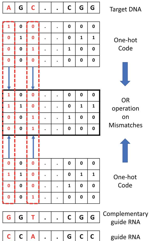
**Fig. 1.** An example on how to encode a sgRNA-DNA sequence pair. The table with thick borders in the middle of the figure shows the final code matrix of a sgRNA-DNA sequence pair, which can be used as the input for CNN modelling
