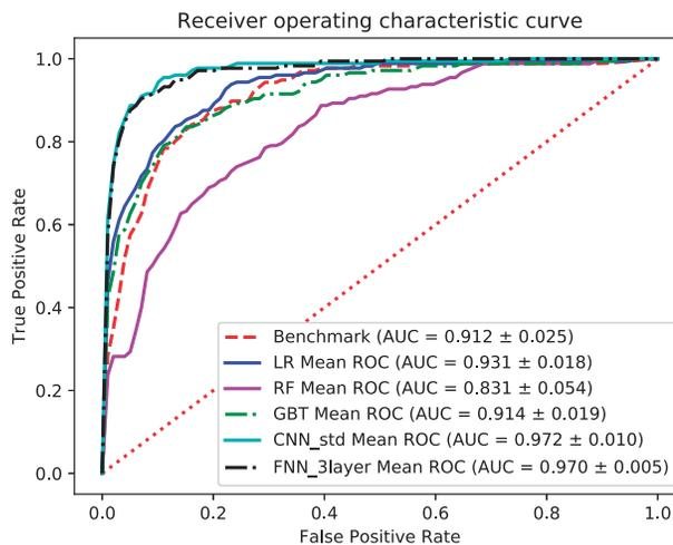
**Fig. 4.** ROC curves of two deep learning models (i.e. FNN\_3layer and CNN\_std) and three traditional machine learning models including LR, RF and GBT. The ROC curve and AUC value of CFD score were regarded as the state-of-arts benchmark on the figure
