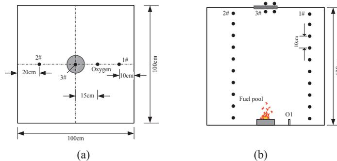
Figure 1. Experimental arrangement: (a) top view, (b) lateral view.
