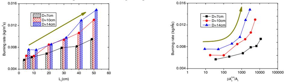
Figure 2(a) Variation in burning rate values with vent sizes, and(b) dimensional horizontal ventilation parameter.
