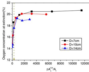
Figure 3 The oxygen concentration at extinction of three different pool fires
