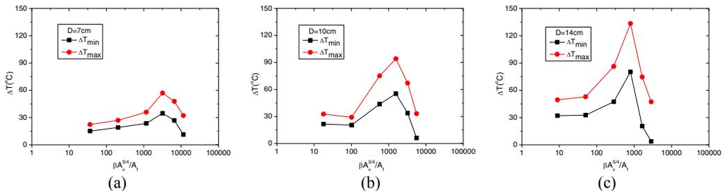
Figure 4 The effect of dimensional horizontal ventilation parameter on temperature difference in the horizontal opening for 7cm (a),10cm (b) and 14cm (c) pool fires.
