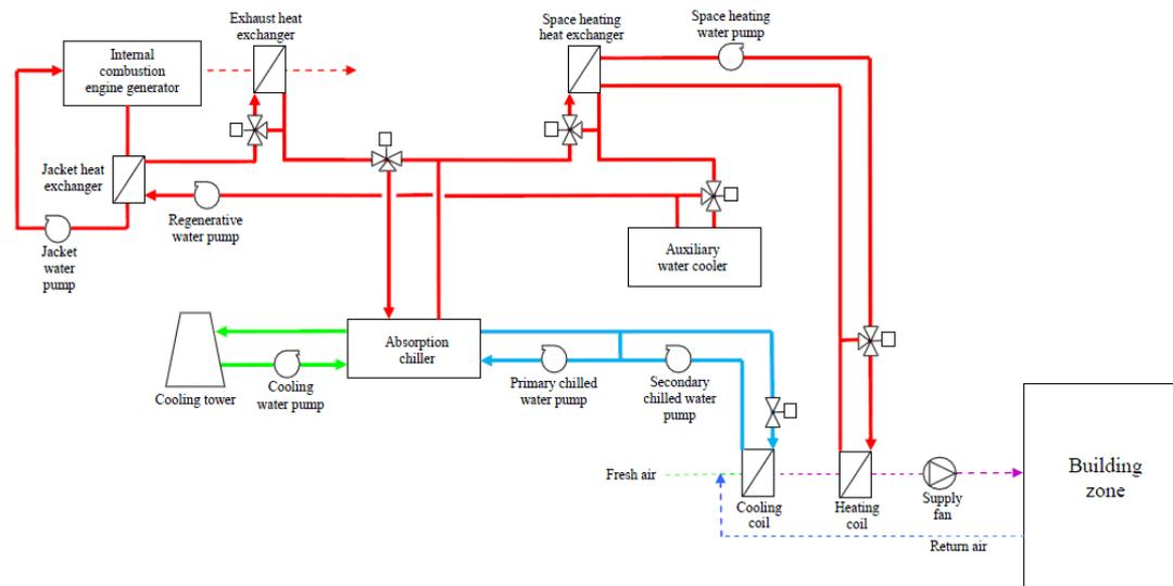
Fig. 1. Schematic diagram of an internal-combustion-engine-primed trigeneration system
