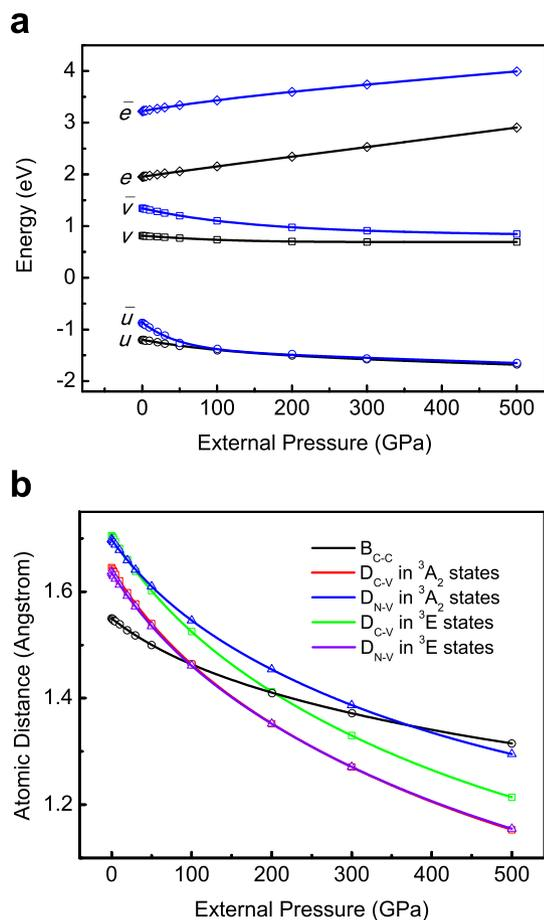
**Figure 3 | Defect levels and atomic configuration under external high pressures.** (a), Energy versus pressure curve for spin-polarized single-electron levels (with respect to the VBM) of the  $N-V^-$  center in the  $^3A_2$  states. (b), Calculated C-C bond length ( $B_{C-C}$ ) in diamond; C-V ( $D_{C-V}$ ) and N-V ( $D_{N-V}$ ) distances of the  $N-V^-$  center under high pressures in  $^3A_2$  and  $^3E$  states.
