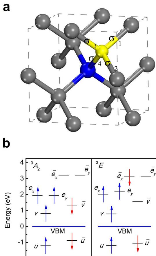
**Figure 1** | Structure of the N-V center in diamond. (a), Atomic structure of the N-V<sup>-</sup> center. The vacancy is indicated by a small yellow ball and the adjacent C and N by gray and blue balls, respectively (b), Electronic structure of the N-V<sup>-</sup> center: the calculated spin-polarized single-electron levels (with respect to the VBM), in <sup>3</sup>A<sub>2</sub> ground states and <sup>3</sup>E excited states.
