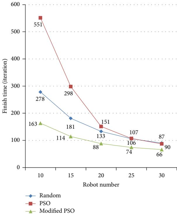
FIGURE 6: The total iteration of different methods. There are 20 obstacle in the map.
