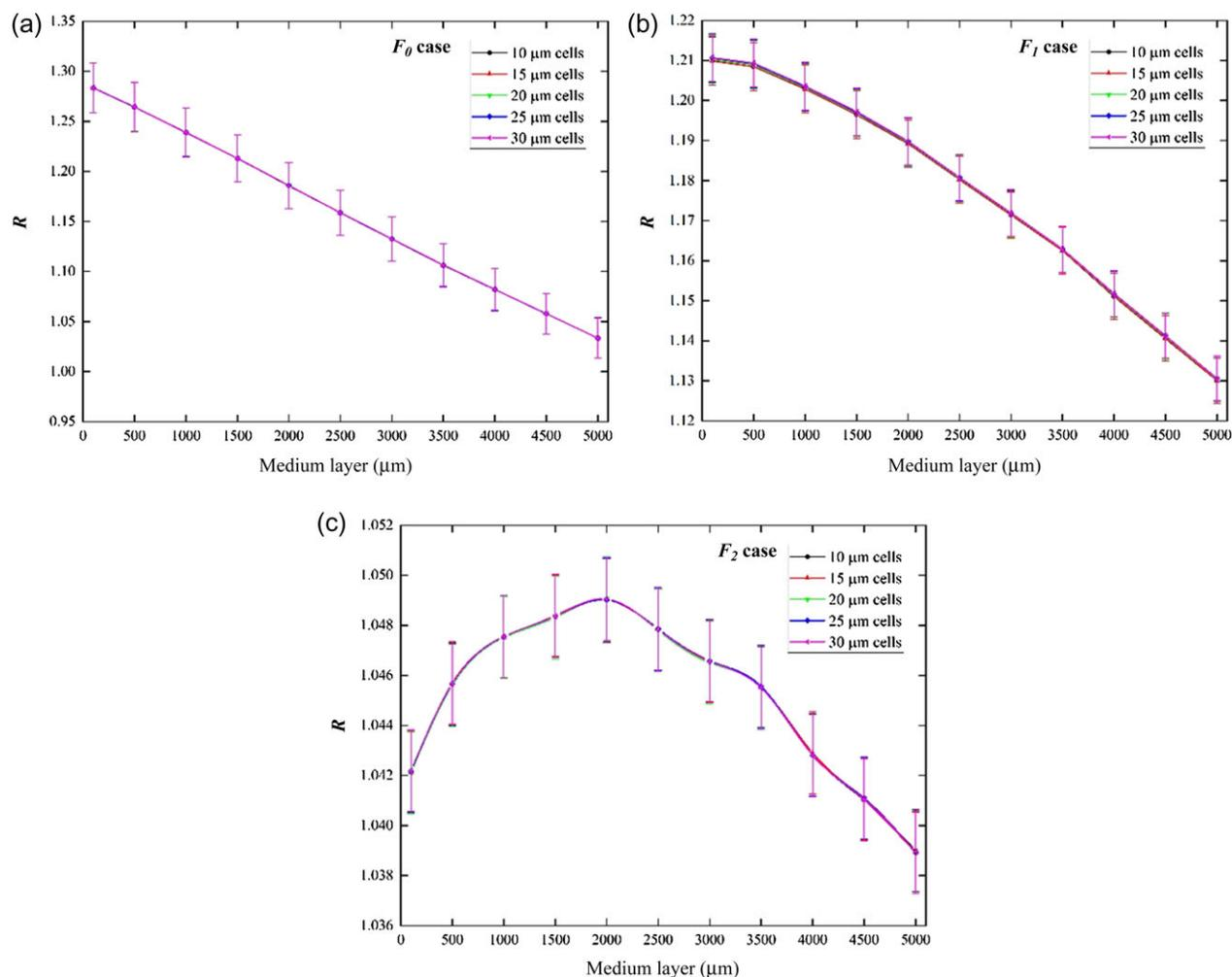
**Fig. 5.** Ratios  $R$  between actual dose absorbed in the cell layer ( $D_A$ ) and dose absorbed in the IOC ( $D_E$ ) for photon energy distributions in the (a)  $F_0$  case, (b)  $F_1$  case and (c)  $F_2$  case. The uncertainties represent the relative errors from Monte Carlo simulations. The average difference in  $R$  for different cell thicknesses is  $\sim 0.000305$ .
