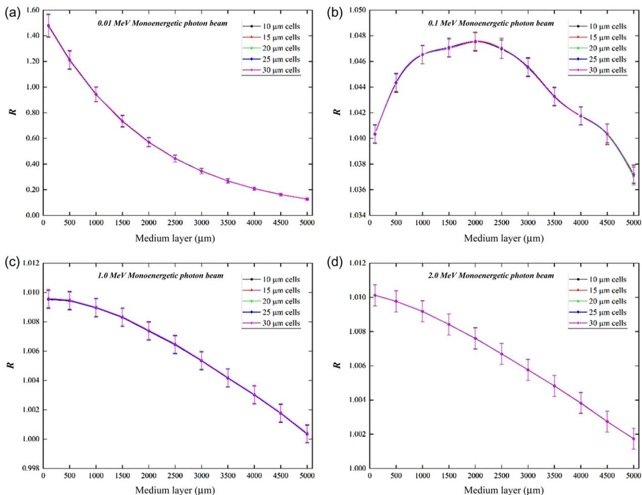
**Fig. 4. Ratios  $R$  between actual dose absorbed in the cell layer ( $D_A$ ) and the dose absorbed in the IOC ( $D_E$ ) for (a) 0.01 MeV, (b) 0.1 MeV, (c) 1 MeV and (d) 2 MeV monoenergetic photon beams. The uncertainties represent the relative errors from Monte Carlo simulations. The average difference in  $R$  for different cell thicknesses is  $\sim 0.000243$ .**
