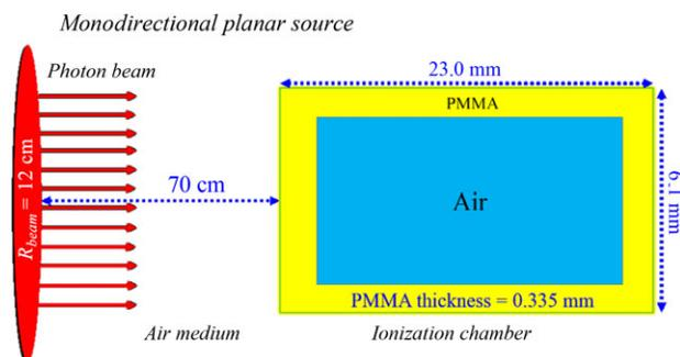
Fig. 2. Schematic diagram showing the photons impinging the ionization chamber model TN 30 013, PTW Farmer® Chamber (IOC) and the sensitive air volume of the IOC in which the energy deposition takes place.
