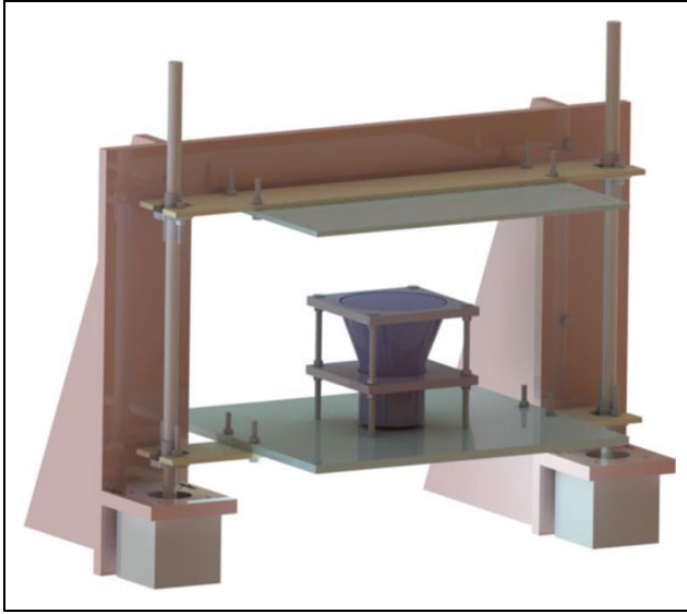
Figure 4. The design of ultrasonic levitation setup in the perspective view.
