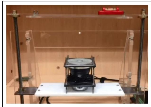
**Figure 6.** Levitation with one bead.
