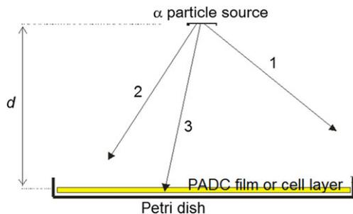
**Fig. 1.** Schematic diagram showing the irradiation of the target (cell layer or PADC film) located on the inner bottom of the Petri dish with the  $^{241}\text{Am}$  source, with  $d$  as the vertical distance between the  $^{241}\text{Am}$  source and the target. The three possible fates for the alpha particles (labeled as 1, 2 and 3) are explained in the text.
