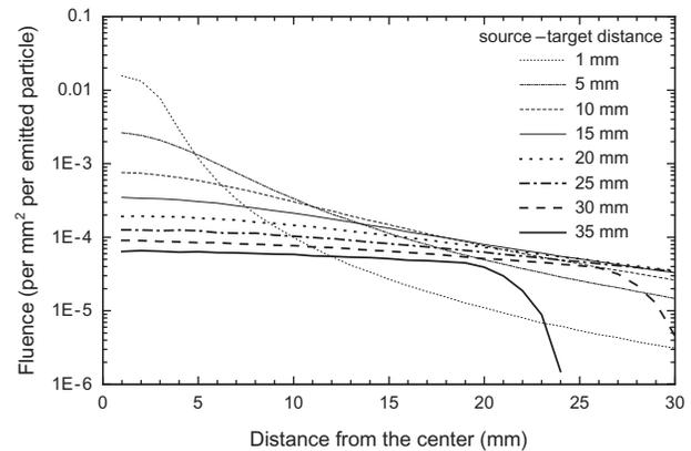
Fig. 4. Relationship between fluence ( $\text{mm}^{-2}$  per emitted alpha particle) and the radial distance from the center of the target, calculated for various source–target distances.
