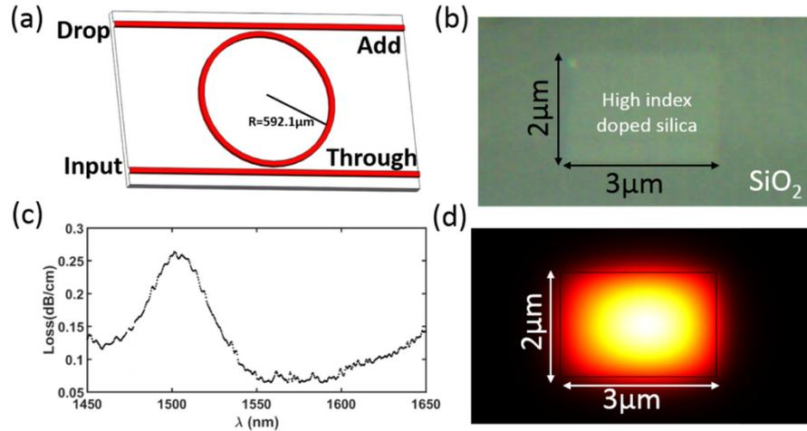
Fig. 1. (a) Schematic illustration of add-drop type MRR. (b) SEM image of the cross section of the MRR. (c) Measured loss parameter versus wavelength. (d) Calculated fundamental TM mode used for generating SC.
