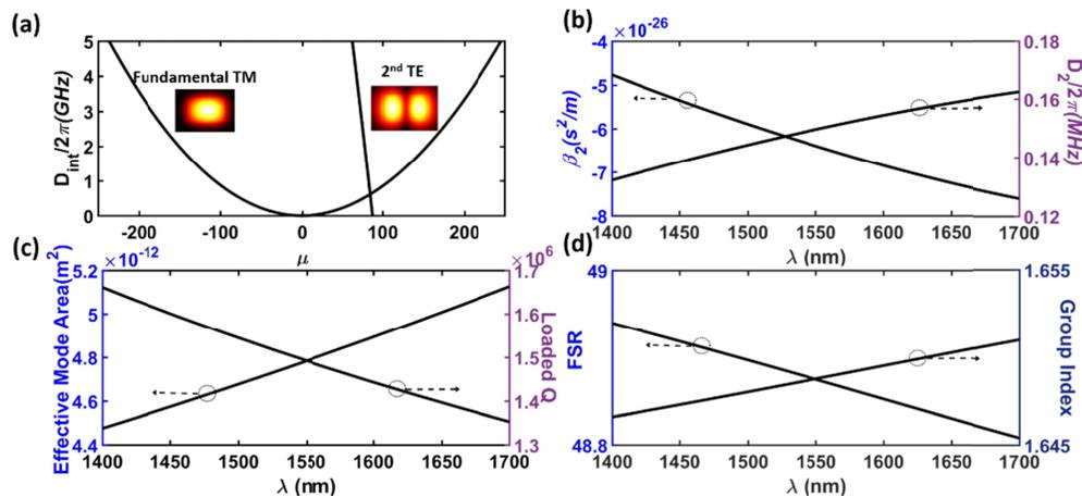
Fig. 2. Calculated major parameters of the MRR. (a) Integrated dispersion curve at pump wavelength (1556.3 nm in experiment), exhibiting perfect parabolic characteristic. The intersection curve belonging to 2nd TE mode induces mode interaction. Insets: calculated optical field of SC-forming and interaction mode. (b) GVD and  $D_2$  curves. (c) Effective mode area and loaded Q value of the MRR. (d) FSR and group refractive group index.
