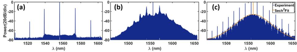
Fig. 4. SC evolution process. (a) Primary comb. (b) MI comb. (c) SC with one soliton out of phase.
