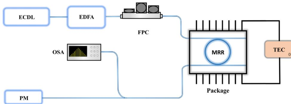
Fig. 3. Experiment set-up of the SC. ECDL: external cavity diode laser. EDFA: erbium doped fiber amplifier. FPC: fiber polarization controller. MRR: micro-ring resonator. TEC: thermoelectric cooler. OSA: optical spectrum analyzer. PM: power meter.
