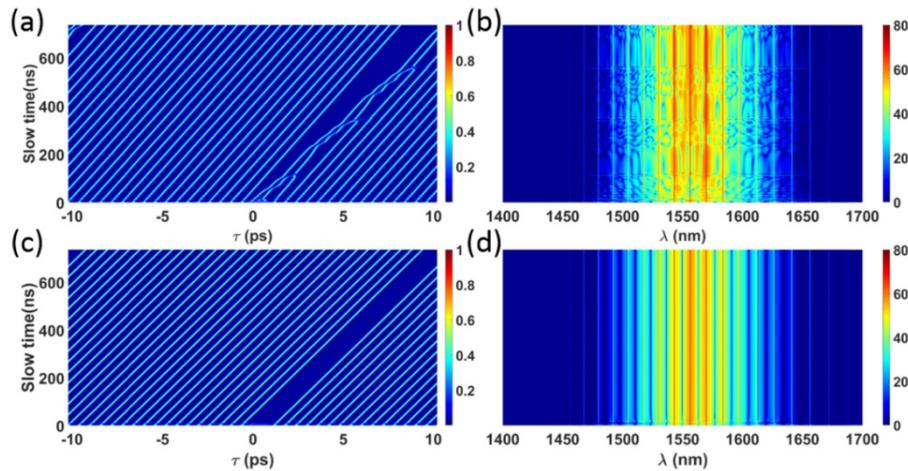
Fig. 5. SC evolution within different condition. Unstable state in (a) time domain and (b) frequency domain with  $\delta = 0.013$  and  $\tau_R = 2.55$  fs. Stable state in (c-d) shows robust evolution with  $\delta = 0.018$  and  $\tau_R = 2.55$  fs.
