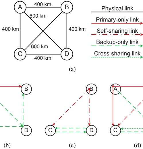
Fig. 1. An example of the shared protection scheme: (a) a four-node fully-mesh network; (b) routing for  $M1 = \langle A; \{B, C\} \rangle$ ; (c) routing for  $M2 = \langle B; \{C, D\} \rangle$ ; and (d) sharing between  $M1$  and  $M2$ .
