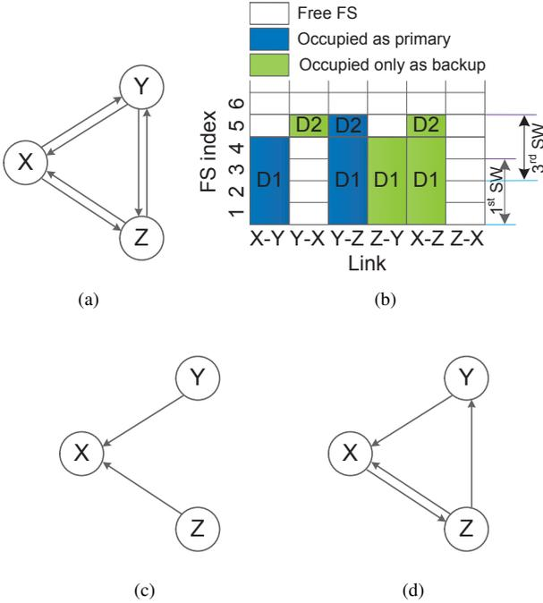
Fig. 2. Illustration for the concepts of SW and SWP: (a) an example network graph; (b) FS usage; (c) a graph  $G_p$  on the first SWP for finding a primary tree for a demand requesting for 3 FSs; (d) a graph  $G_b$  of the first SWP for finding the backup paths for a demand requesting for 3 FSs.
