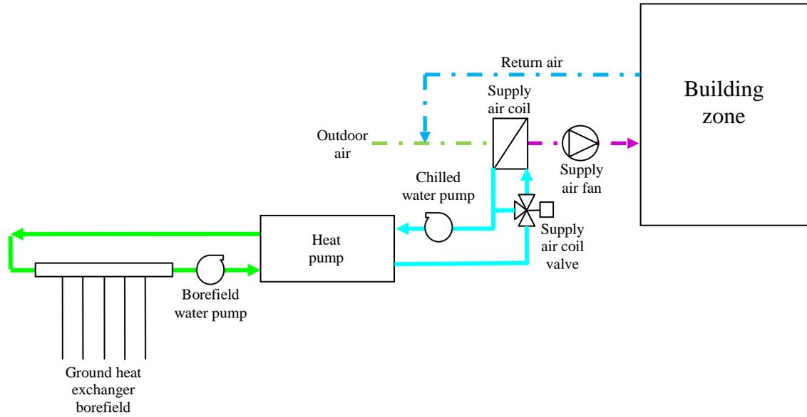
Fig. 5. Schematic diagram of ground-source heat pump system for building cooling.
