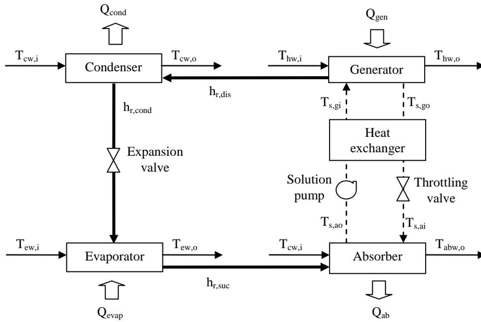
Fig. 3. Schematic diagram of a single-effect lithium bromide absorption chiller [25].
