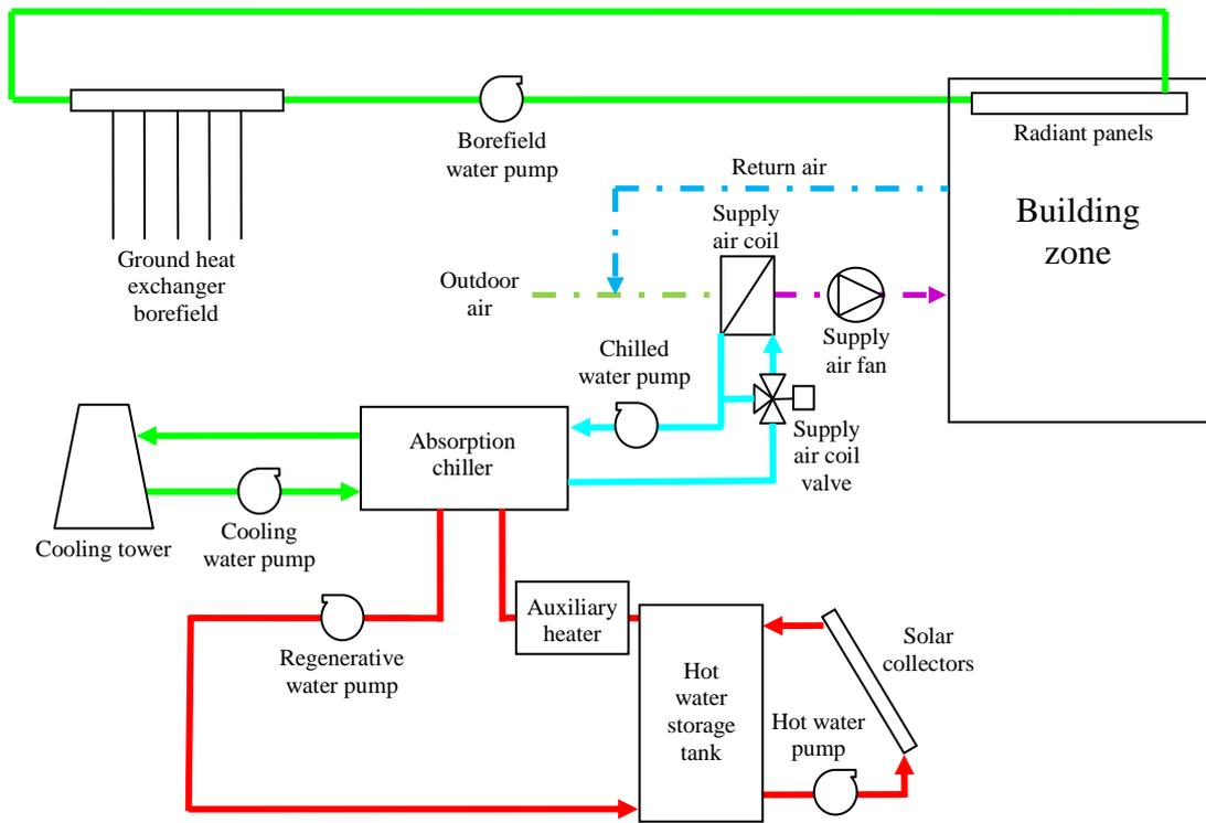
Fig. 1. Schematic diagram of hybrid renewable cooling system for building application.
