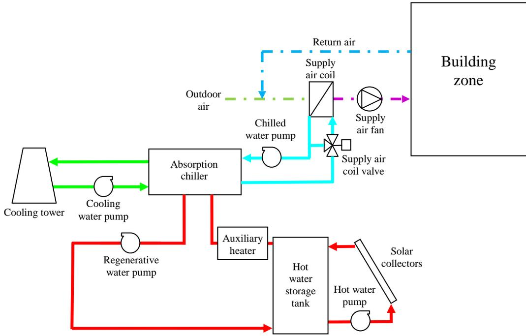
Fig. 4. Schematic diagram of solar absorption cooling system.
