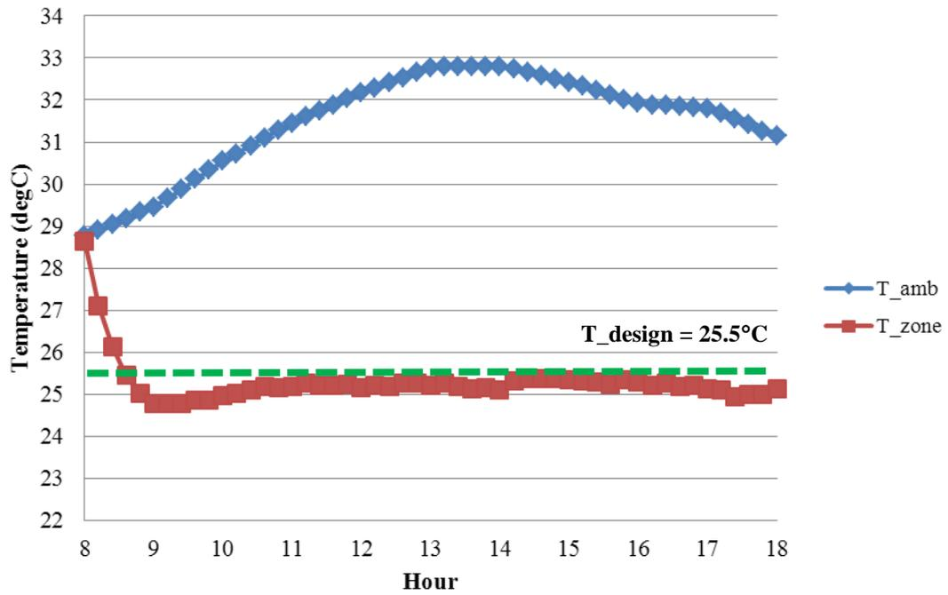
Fig. 8. Daily temperature profile of the HRCS with PCB and reduced capacity of absorption cooling part on the hottest day (T\_amb: Ambient temperature; T\_zone: Zone temperature; T\_design: Indoor design temperature).
