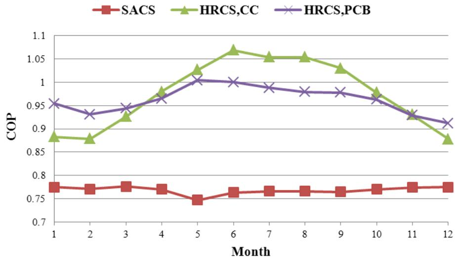
Fig. 7. Comparison of the monthly-averaged *COP* for the various solar cooling systems.
