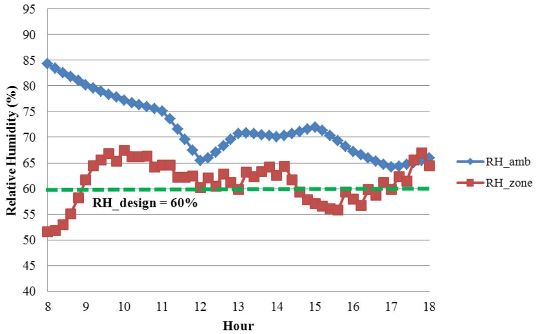
Fig. 9. Daily relative humidity profile of the HRCS with PCB and reduced capacity of absorption cooling part on the hottest day (RH\_amb: Ambient relative humidity; RH\_zone: Zone relative humidity; RH\_design: Indoor design relative humidity).
