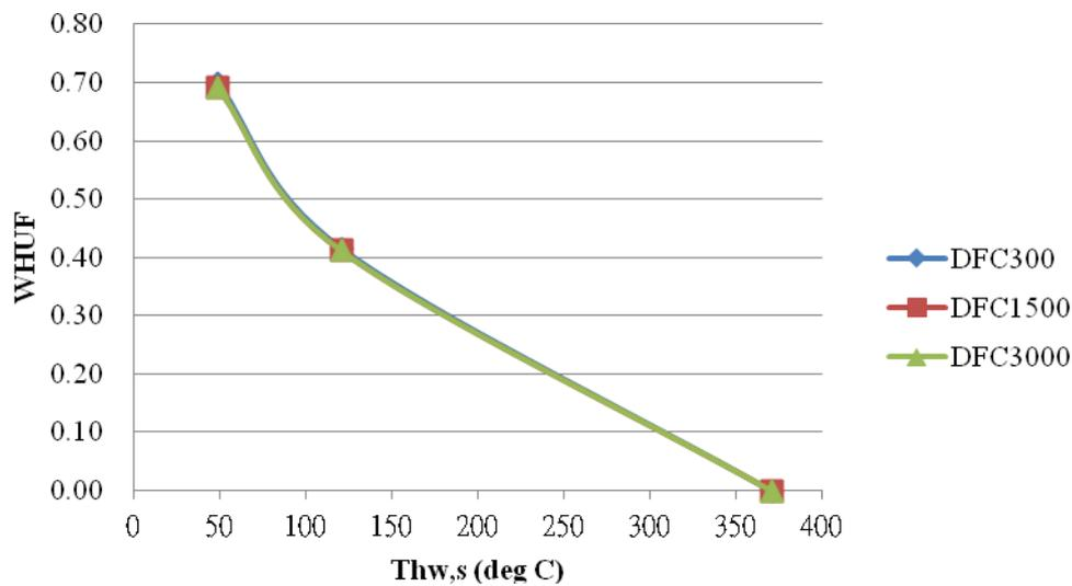
Fig. 4. Variation of  $WHUF$  with  $T_{hw,s}$  for various SOFC models.
