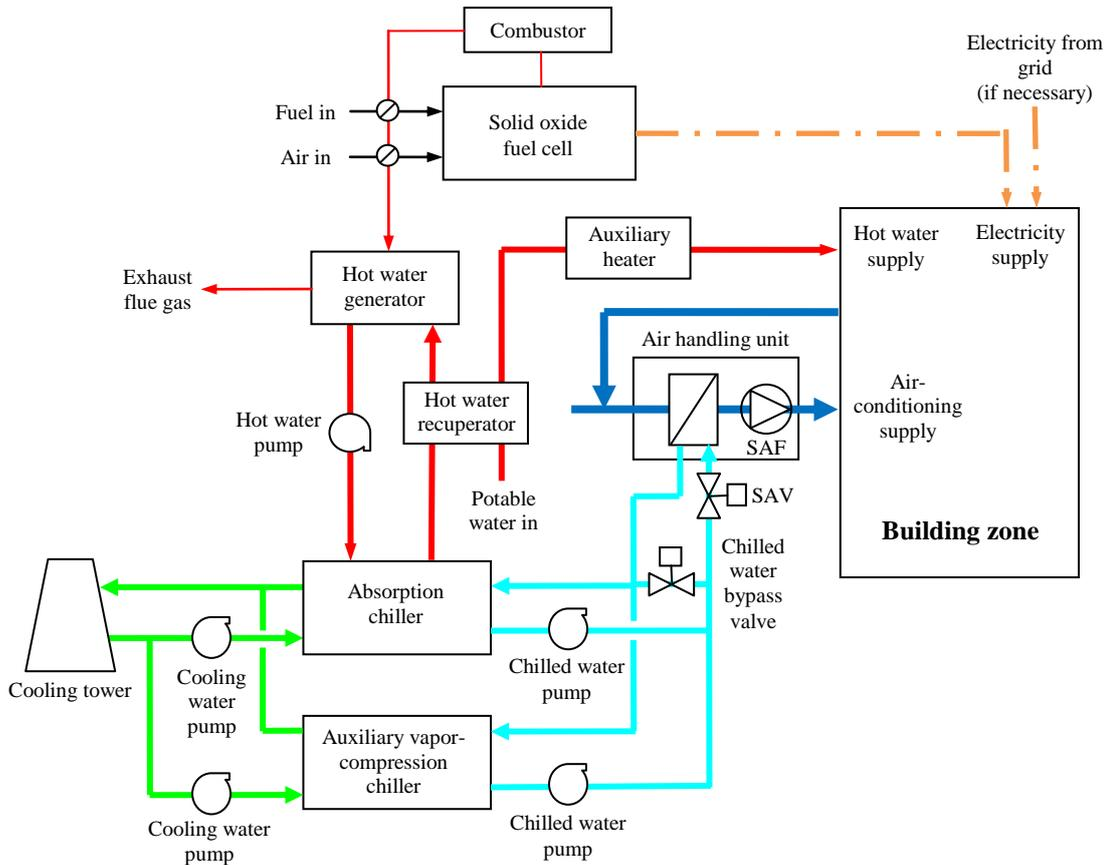
Fig. 1. Schematic diagram of SOFC-trigeneration system.
