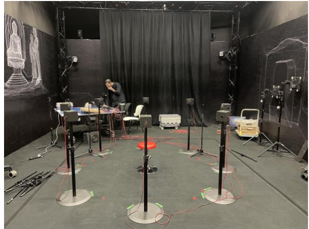
Figure 1. OAT in an octophonic (8.1) configuration during listening tests.
