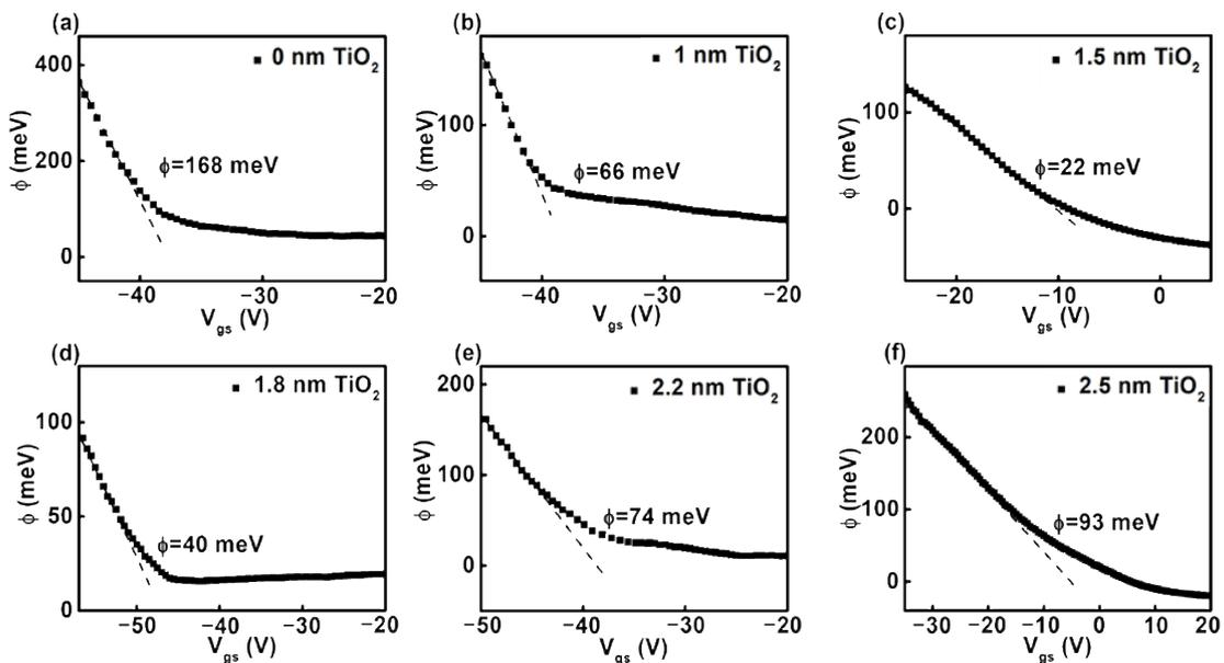
Figure 5. (a–f) Effective Schottky barrier heights as a function of gate overdrive for various TiO<sub>2</sub> thicknesses.
