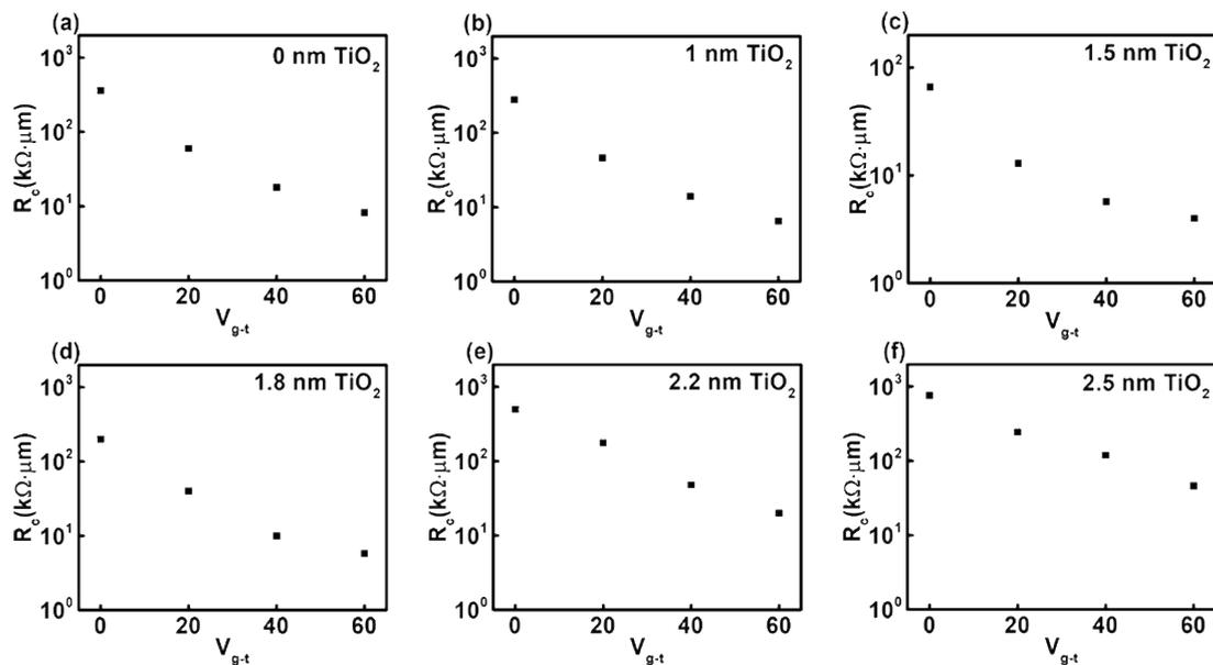
Figure 4. (a–f) Contact resistances for various TiO<sub>2</sub> thicknesses.
