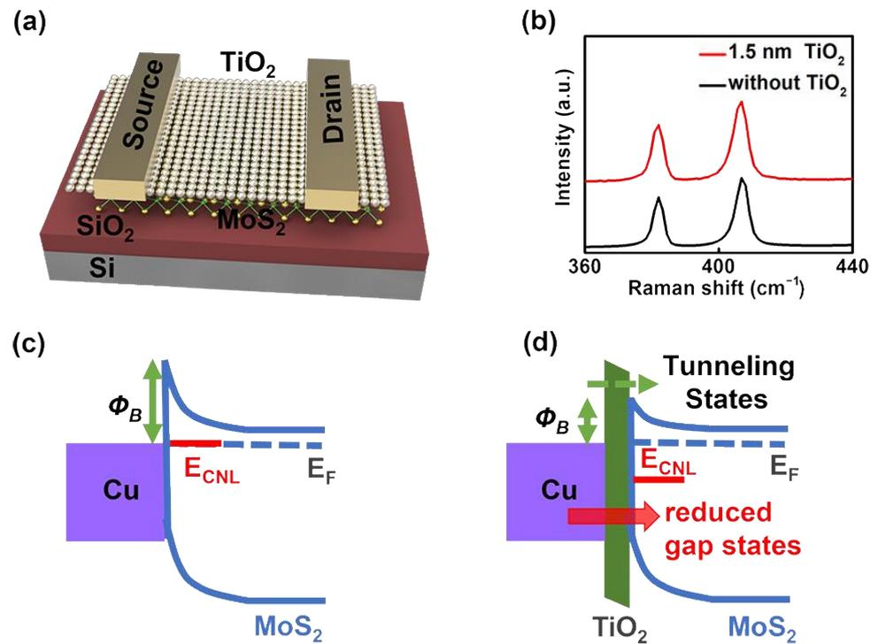
**Figure 2.** (a) Fabrication schematic of the MoS<sub>2</sub> FETs with a TiO<sub>2</sub> interlayer; (b) Raman scattering spectra of the multilayer MoS<sub>2</sub> without and with the TiO<sub>2</sub> layer; (c,d) band diagrams of the MS structure and MIS structure.
