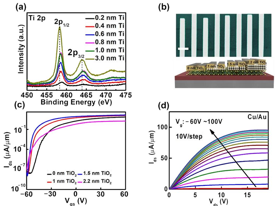
**Figure 3.** (a) Ti 2p spectra of TiO<sub>2</sub> with different thicknesses; (b) SEM image and schematic diagram of the back-gated Cu-TiO<sub>2</sub>-MoS<sub>2</sub> FETs with various TiO<sub>2</sub> thicknesses (0, 1, 1.5 and 2.2 nm) (scale bar = 5 μm); (c) transfer characteristics of the devices for various TiO<sub>2</sub> thicknesses with *L* being 3 μm and *V<sub>ds</sub>* being 1 V; (d) output characteristics of the Cu-TiO<sub>2</sub>-MoS<sub>2</sub> FETs.
