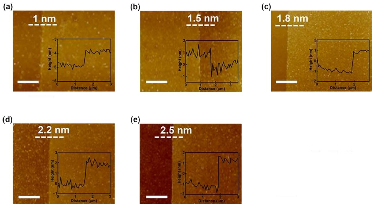
**Figure 1.** (a–e) AFM images of the TiO<sub>2</sub> interlayers with different thicknesses on the SiO<sub>2</sub> substrate. The thicknesses of Ti are 0.2, 0.4, 0.6, 0.8 and 1 nm; these correspond to thicknesses of TiO<sub>2</sub> of 1, 1.5, 1.8, 2.2 and 2.5 nm, respectively. The scale bar is 2 μm.
