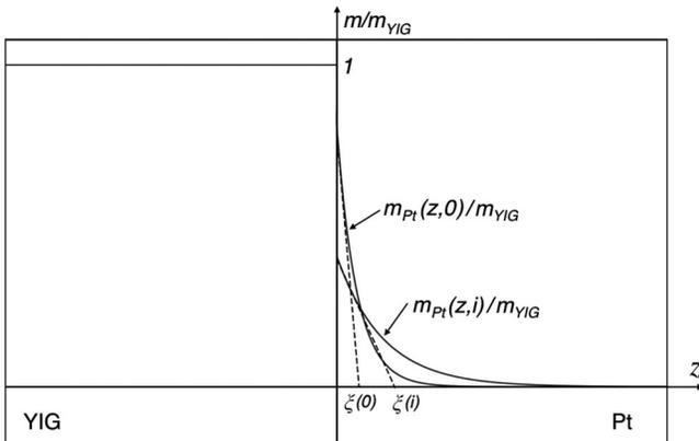
FIG. 4. Schematic representation of the magnetic proximity effect in YIG/Pt bilayers.
