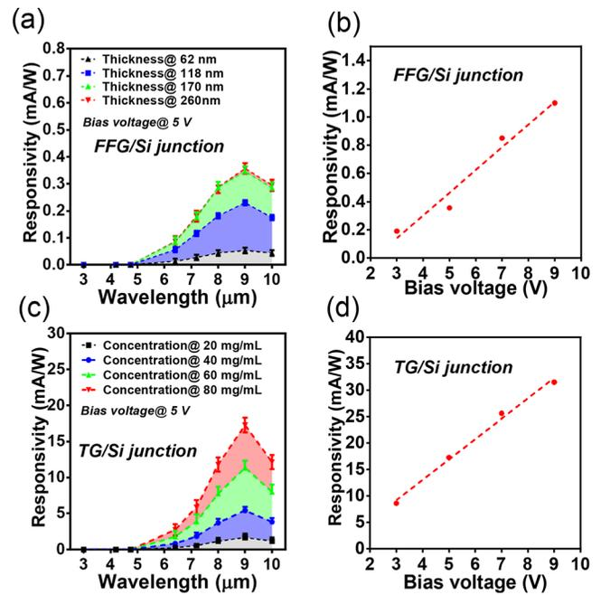
FIG. 3. (a) The spectral responsivity as a function of the thickness of HgSe CQD films ( $N=8$ ). (b) Bias voltage-dependent responsivity at a wavelength of 9.0  $\mu\text{m}$  of the FFG/Si junction. (c) The spectral responsivity as a function of the concentration of HgSe CQD solution ( $N=8$ ). (d) Bias voltage-dependent responsivity at a wavelength of 9.0  $\mu\text{m}$  of the TG/Si junction.
