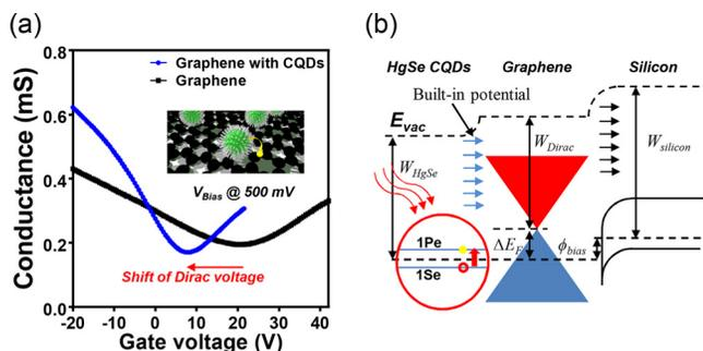
FIG. 4. (a) Gate-dependent transfer curve of graphene with/without HgSe quantum dots. (b) Energy band diagram of the CQD-graphene/silicon heterojunction.
