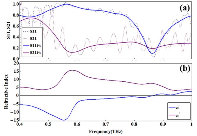
FIG. 5. (a) S11 and S21 of PDLC-TFMM at 0 V bias before and after time window is applied. The dashed and dotted lines represent original S11 and S21. Significant FP effect is observed in original S21. Solid lines are S11 (S11tw) and S21 (S21tw) with time window applied. (b) Real and imaginary refractive index of PDLC-TFMM at 0 V bias is calculated based on S11tw and S21tw.
