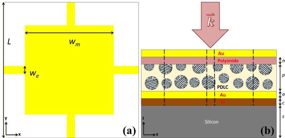
FIG. 1. PDLC-TFMM unit cell: (a) overhead view of unit cell with  $L = 150 \mu\text{m}$ ,  $w_m = 115 \mu\text{m}$ , and  $w_e = 10 \mu\text{m}$ ; (b) cross section of the unit cell, with thicknesses of  $m = 1.5 \mu\text{m}$ ,  $p = 10 \mu\text{m}$ ,  $a = 0.25 \mu\text{m}$ ,  $c = 5 \text{ nm}$ , and  $s = 1 \text{ mm}$ .
