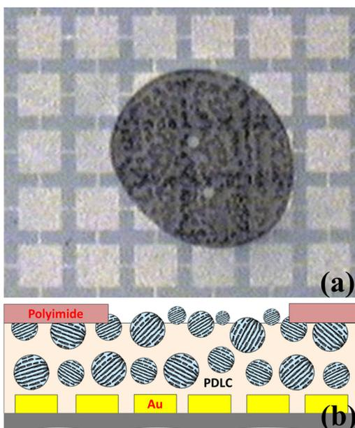
FIG. 2. PDLC with and without polyimide skin layer: (a) overhead view of the liquid crystal droplets accumulating at center of the device where skin layer is removed; (b) cross section of the PDLC fabricated on top of the fishnet pattern and silicon substrate.
