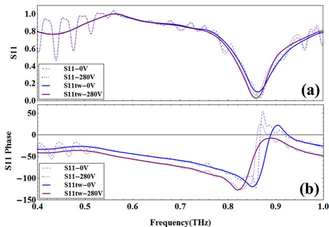
FIG. 6. Tunability of PDLC-TFMM at 0 V and 280 V bias can be seen in (a) S11 and (b) S11 phase. The dashed and dotted lines represent original S11 at 0 V and 280 V. Significant FP effect can be seen in the lower frequency range (0.4 to 0.55 THz) but the effect can be removed by time window technique.
