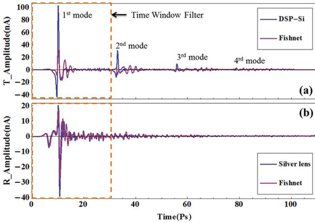
FIG. 4. Time domain signals of PDLC-TFMM at 0 V bias: (a) transmission measurement with time window applied to remove multiple internal reflections from DSP-Si; (b) reflection measurement with time window applied. Higher FP modes decay faster compared to transmission mode.
