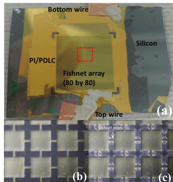
FIG. 3. PDLC-TFMM testing sample: (a) perspective view of testing sample; (b) microscopic view of PLDC-TFMM at 0 V; (c) microscopic view of PLDC-TFMM at 280 V.
