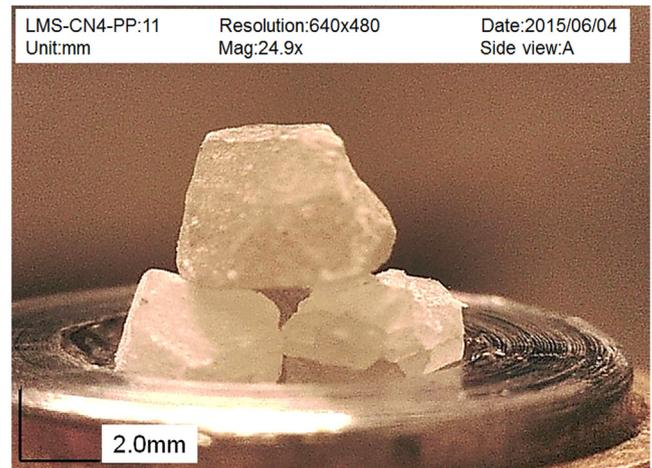
Fig. 6. Flat-to-flat contacts between LMS particles.
