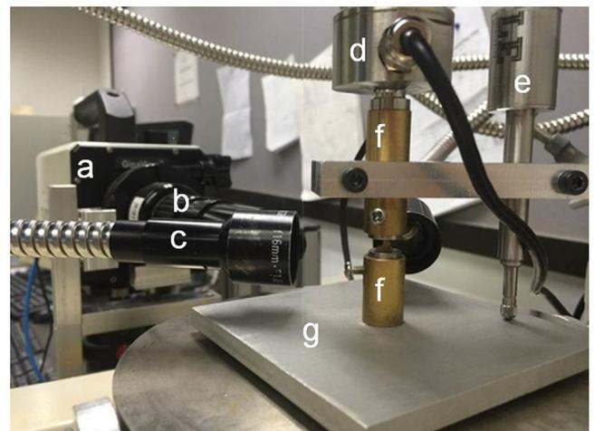
Fig. 1. Equipment for multi-axial crushing tests: (a) high speed camera; (b) microscope lens; (c) additional lighting system with focussing lenses; (d) load cell; (e) LVDT; (f) brass wells containing steel mounts; and (g) base support resting on ball bearings.
