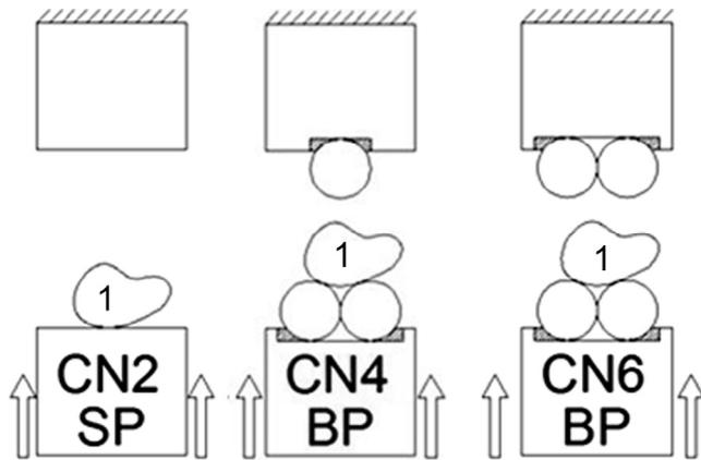
Fig. 2. Schematic representation of multi-contact crushing tests for particles tested between hardened steel mounts (SP), between 4 steel balls (CN4-BP), and between 6 steel balls (CN6-BP).
