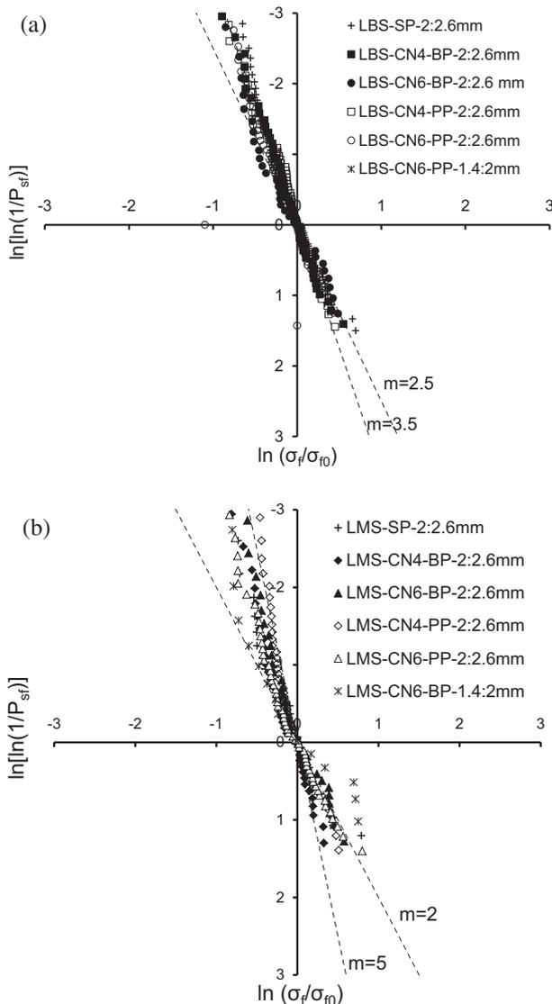
Fig. 15. The m-modulus of tested sands: (a) LBS specimens and (b) LMS specimens.
