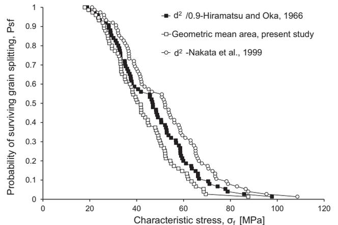
Fig. 5. The effect of the failure area on the strength of the LBS particles crushed between two hardened steel mounts, i.e., LBS-SP. The geometric mean area has been adopted in this study.
