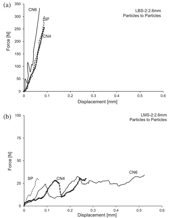
Fig. 14. Force-displacement relationship of (a) LBS (present study) and (b) LMS (redrawn from Todisco et al., 2015) particles.
