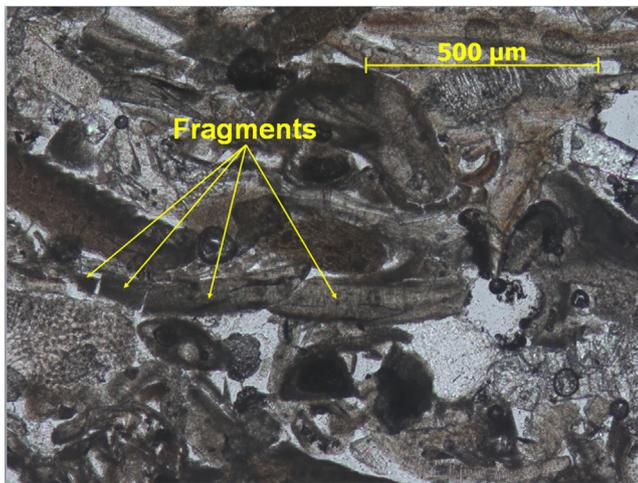
Fig. 21. Example of fragments of particle confined to their initial position (redrawn from Bandini and Coop, 2011).
