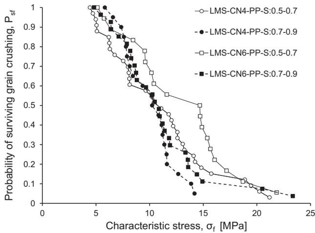
Fig. 7. Effect of sphericity on strength of LMS particles.
