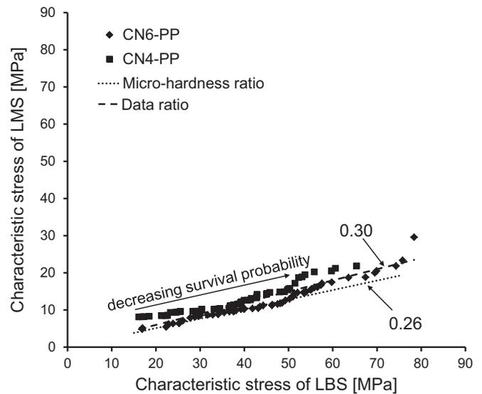
Fig. 11. Hardness relationship obtained from characteristic stress of LBS and LMS specimens crushed in CN4-PP and CN6-PP configurations.
