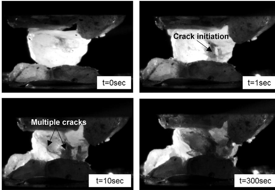
Fig. 10. Example of crushing mechanism of LMS particles tested in CN6-PP configuration.
