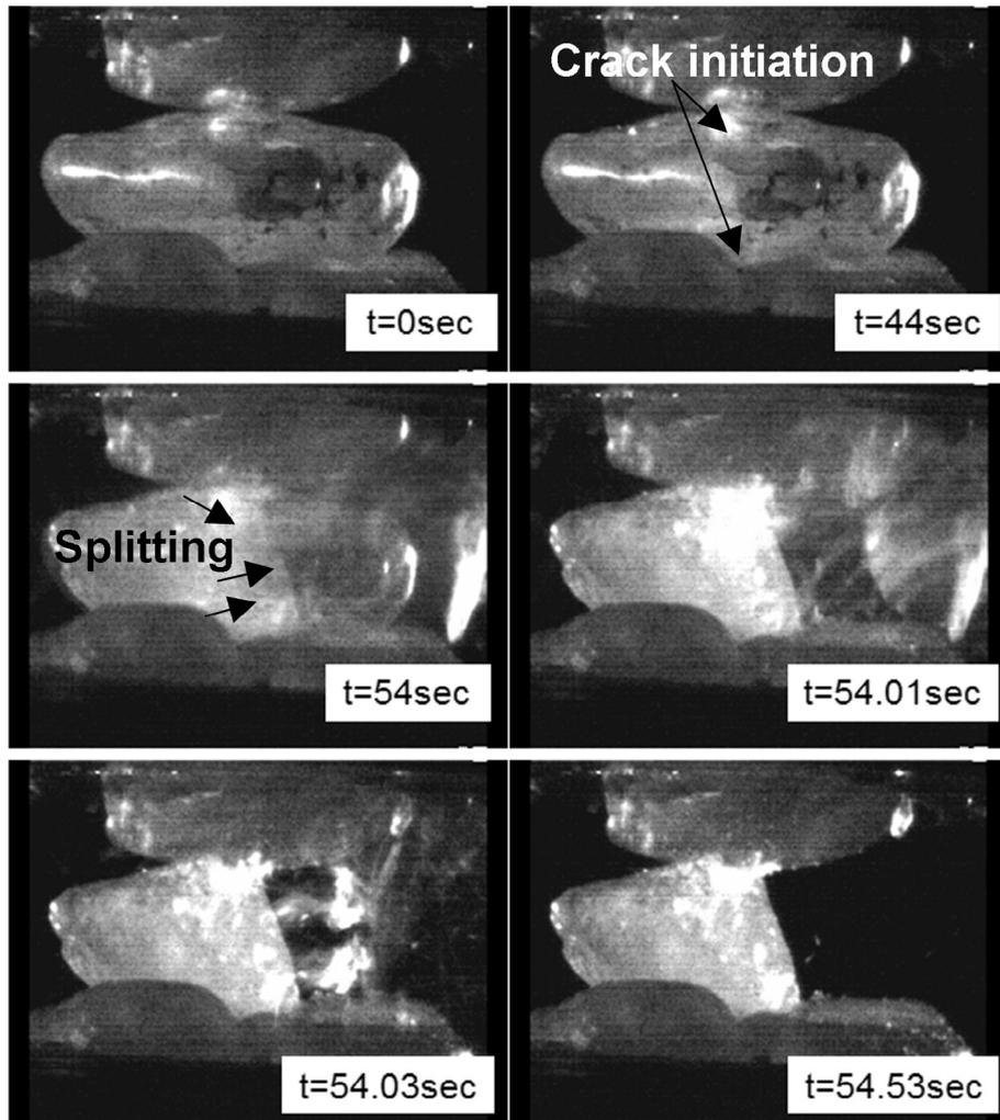
Fig. 18. Splitting crushing mechanism of LBS particle tested in CN4-PP configuration.
