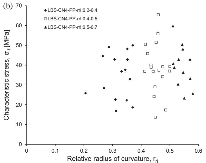
Fig. 9. Effect of local roundness parameter,  $r_{rl}$ , on LBS particles: (a) probability of surviving grain crushing and (b) relationship between characteristic stress and  $r_{rl}$ .
