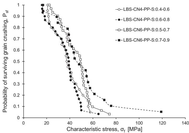
Fig. 8. Effect of sphericity on strength of LBS particles.
