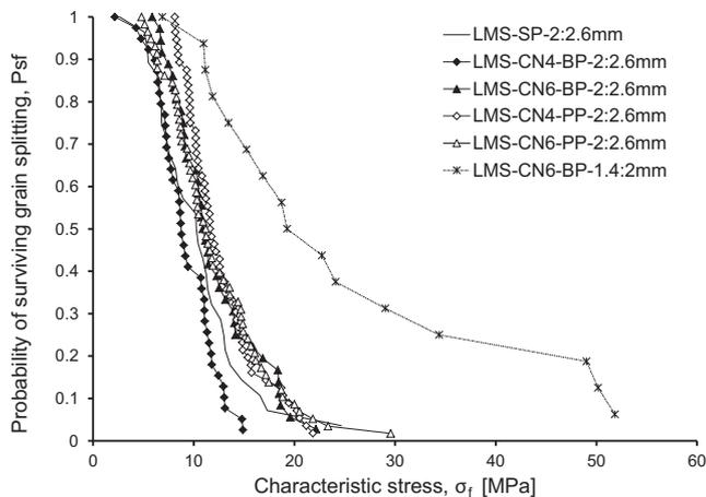
Fig. 13. Survival probability curves of LMS for different support particles.
