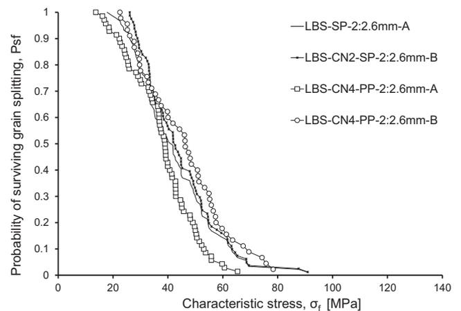
Fig. 16. Probabilities of survival of LBS particles for which crack initiation did not occur near top contact. Data refer to SP and CN4-PP configurations. (A all data and B with failures near top contact eliminated.)
