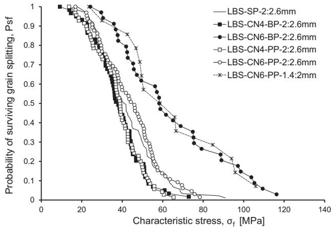
Fig. 12. Survival probability curves of LBS particles for different support particles.
