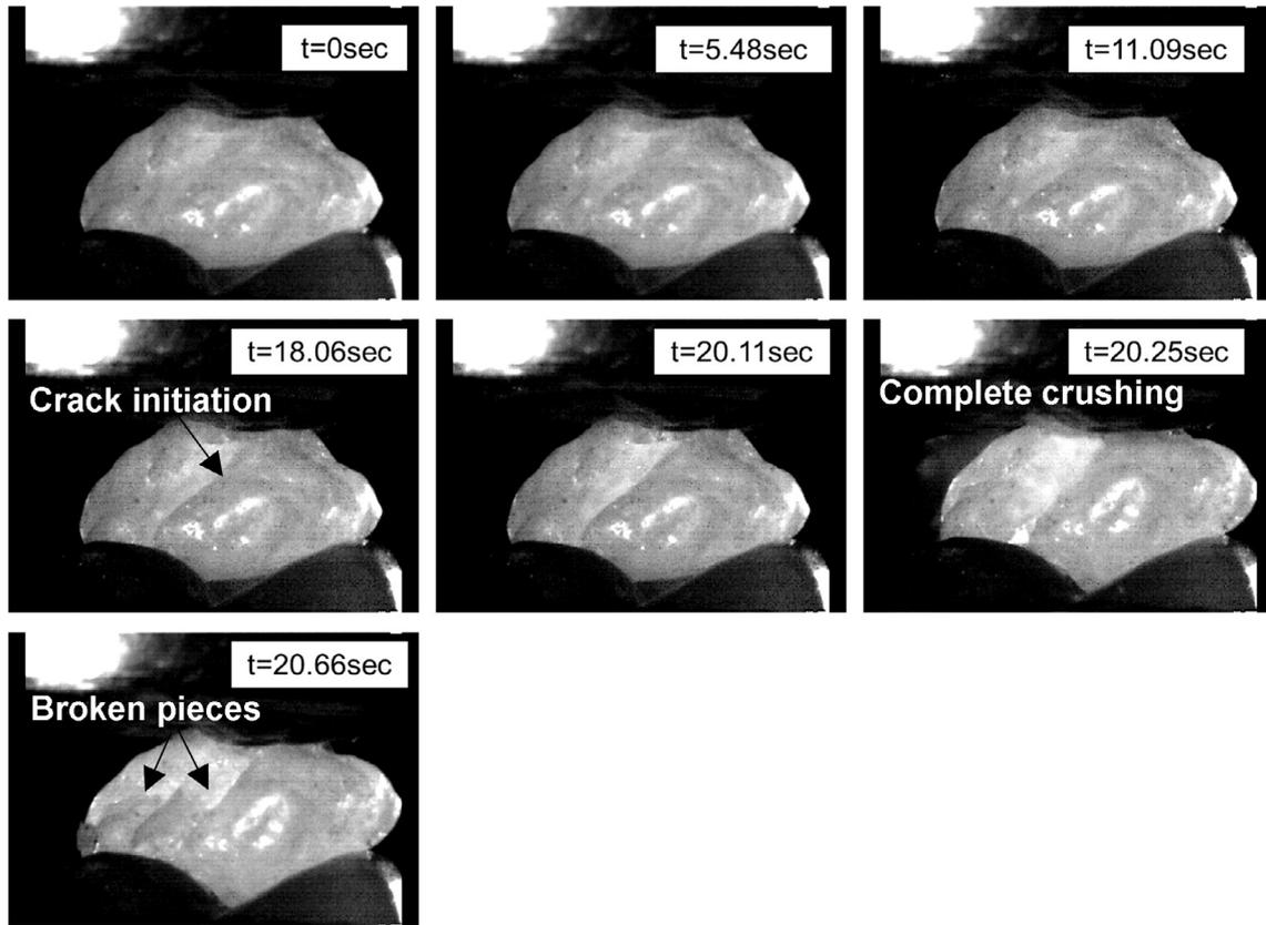
Fig. 20. Splitting crushing mechanism of LBS particle tested in CN6-PP configuration.
