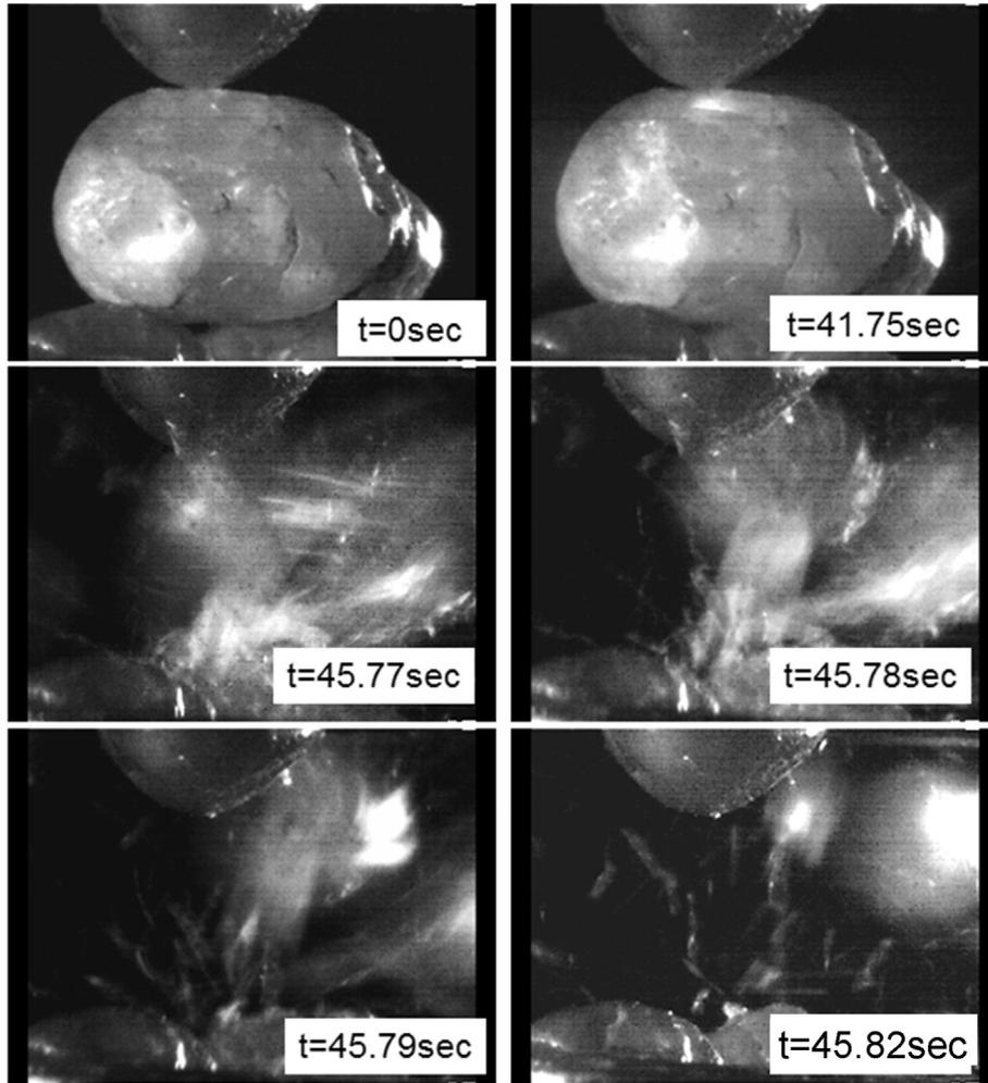
Fig. 19. Fragmentation crushing mechanism of LBS particle crushed between 4 particles.
