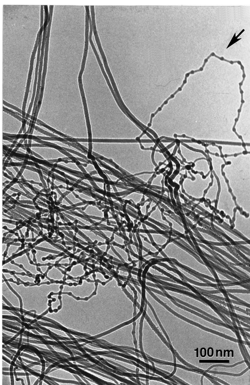
FIG. 1. TEM image showing two major morphologies of Si nanowires.
