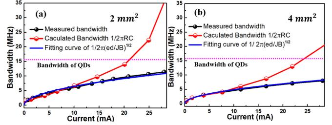
Fig. 8. Variations in the measured bandwidth and the bandwidth calculated from the  $RC$  time constant with the injection current for (a) 2-mm<sup>2</sup> QLED and (b) 4-mm<sup>2</sup> QLED.
