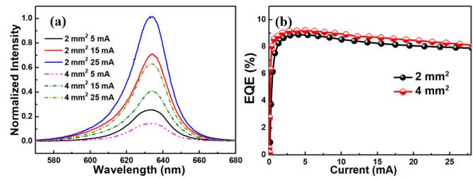
Fig. 5. (a) Normalized emission spectra of the QLED measured at various injection currents and (b) variation in the EQE of the QLED with the injection current for the 2- and 4-mm<sup>2</sup> QLEDs.
