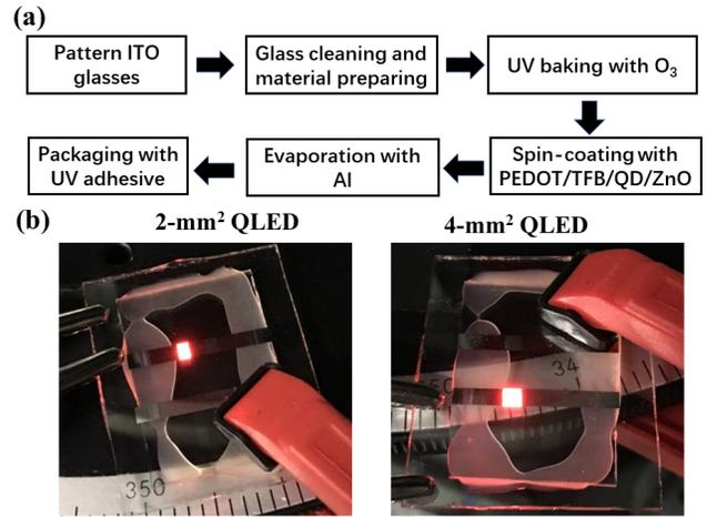
Fig. 2. (a) Steps in the fabrication process of QLED and (b) photographs of a  $2$ - and  $4$ -mm<sup>2</sup> QLED under test.
