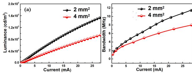
Fig. 9. Comparison of (a) luminance and (b) bandwidth characteristics of the 2- and 4-mm<sup>2</sup> QLEDs.
