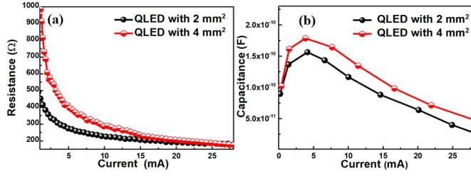
Fig. 7. Variations in (a) resistance and (b) capacitance values with the injection current measured for the 2- and 4-mm<sup>2</sup> QLEDs.
