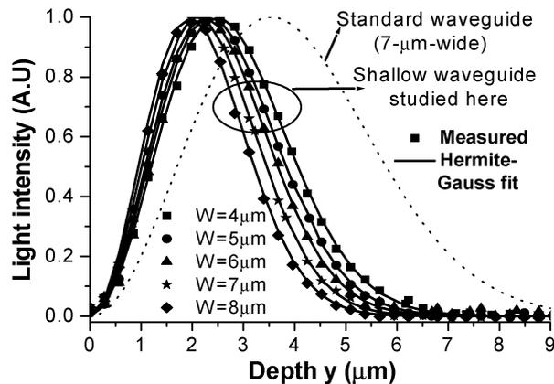
Fig. 2. Measured (scattered symbols) and Hermite–Gauss-fitting (solid lines) field depth profiles of TM modes guided in the strip waveguides with different initial Ti-strip widths. For comparison, the field profile of the TM mode guided in a conventional waveguide is also shown (dotted plot).
