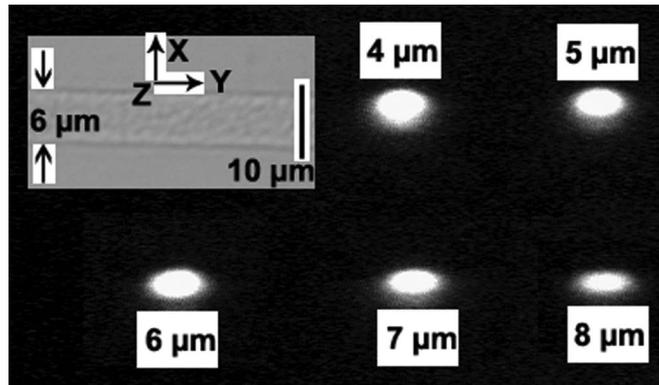
Fig. 1. Morphology image of 6- $\mu\text{m}$ -wide shallow Ti:LN strip waveguide (left upper corner) and near-field patterns of TM mode guided in the 4, 5, 6, 7, and 8- $\mu\text{m}$ -wide waveguides at 1.5- $\mu\text{m}$  wavelength.
