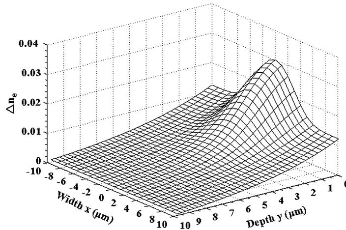
Fig. 5. Surface plot of 2-D Ti<sup>4+</sup>-induced extraordinary index increment in the 6- $\mu\text{m}$ -wide shallow strip waveguide.
