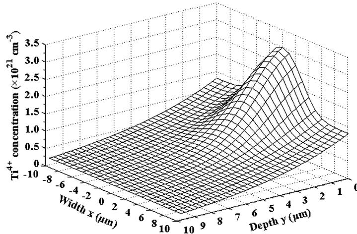
Fig. 4. Surface plot of 2-D  $\text{Ti}^{4+}$ -concentration in the 6- $\mu\text{m}$ -wide shallow strip waveguide.
