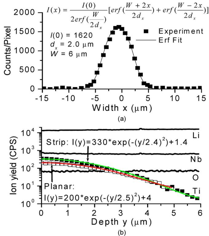
Fig. 3. (a) Surface  $^{48}\text{Ti}$  profile (full squares) of the  $6\text{-}\mu\text{m}$ -wide Ti:LN strip waveguide. (b) Depth profiles of  $^6\text{Li}$ ,  $^{93}\text{Nb}$ ,  $^{16}\text{O}$ , and  $^{48}\text{Ti}$  (full squares) in same strip waveguide. The open squares denote the  $\text{Ti}^{4+}$  profile in the planar waveguide area. The colored curves represent the Gaussian fitting results.
