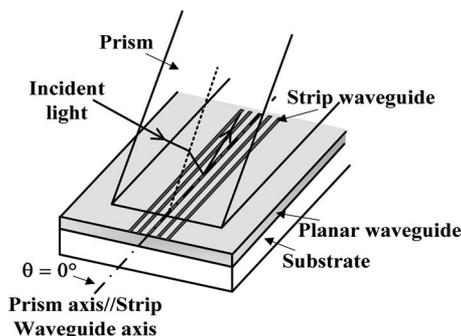
Fig. 2. Schematic of the characterization in the case where the strip waveguide axis is aligned parallel to the prism axis.
