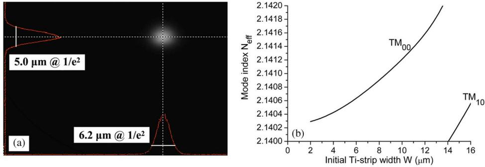
Fig. 5. (a) Near-field pattern of TM-polarized single-mode guided in the strip waveguide of the special waveguide structure at 1.5- $\mu\text{m}$  wavelength. (b) Calculated mode index (at 1.5- $\mu\text{m}$  wavelength) versus initial Ti-strip width  $W$ .
