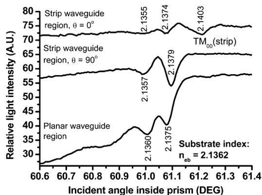
Fig. 4. Patterns of relative intensity of TM-polarized 1553-nm light (reflected from the surface of the strip waveguide array or the planar waveguide area) measured as a function of the incident angle inside the prism.
