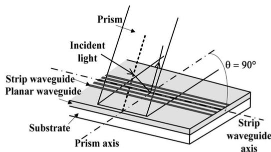
Fig. 3. Schematic of the characterization in the case where the strip waveguide axis is aligned perpendicular to the prism axis.
