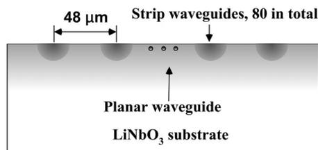
Fig. 1. Schematic of the cross section of an array of 80 8- $\mu\text{m}$ -wide 48- $\mu\text{m}$ -separated Ti:LN strip waveguides embedded in a Ti:LN planar waveguide.
